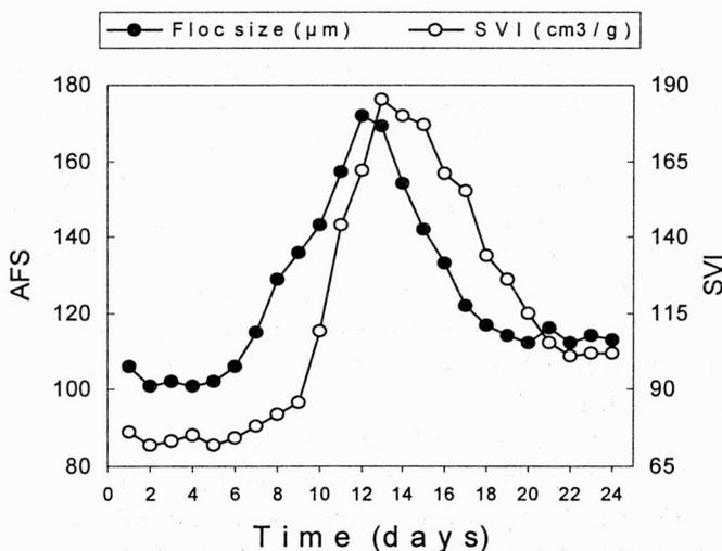
Fig. 1. Time delay of the sludge volume index (SVI) in relation to average floc size (AFS) for bidirectional changes in organic loading; Series II
