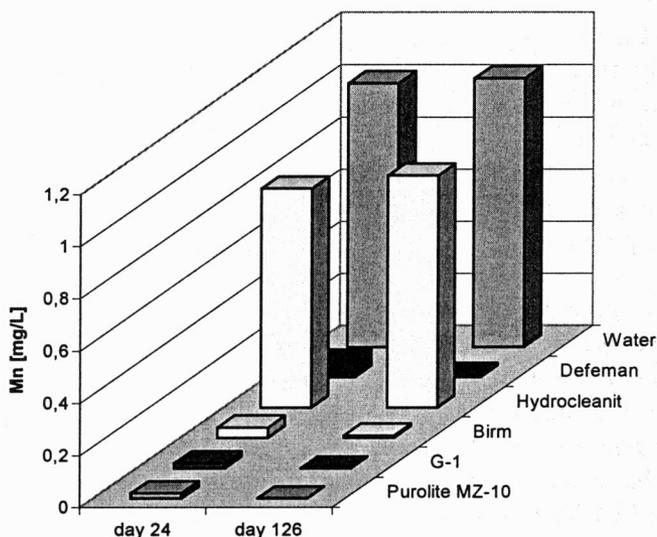
Fig. 2. Manganese concentration in filtrate in chosen days of filtration system operation
