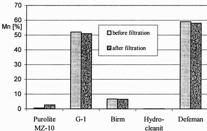
Fig. 4. Manganese percent in active beds before and after filtration process
