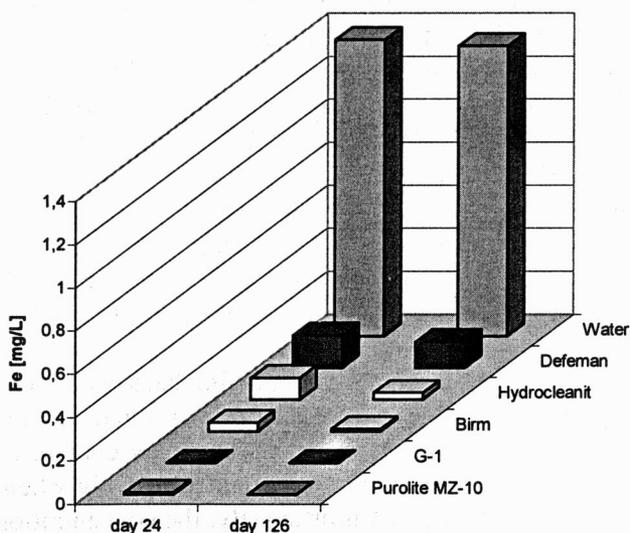
Fig. 3. Iron concentration in filtrate during chosen days of filtration system operation
