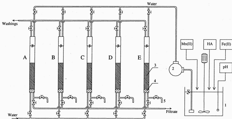
Fig. 1. Experimental set-up: 1 – raw water tank, 2 – dosing pump, 3 – filtration layer (active mass), 4 – supporting layer, 5 – point of taking samples, A – filtration column with the Purolite MZ-10 filler, B – filtration column with the G-1 filler, C – filtration column with the Birm filler, D – filtration column with the Hydrocleanit filler, E – filtration column with the Defeman filler
