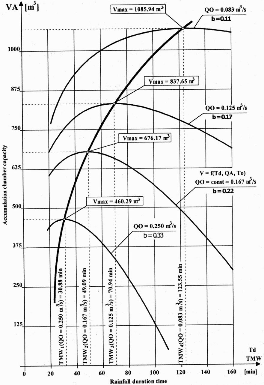
Fig. 5. An example of the result of sewage storage simulation in two-chamber reservoir of the CONTRACT type
