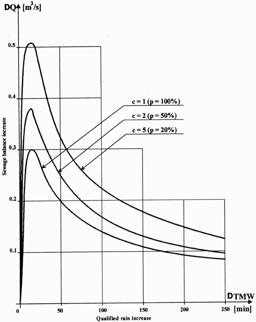
Fig. 4. Diagram of sewage balance for variable qualified time and assumed reliability degree of two-chamber storage reservoir operation
