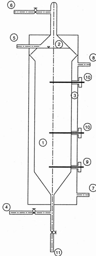
Fig. 2. Scheme of the UASB reactor
