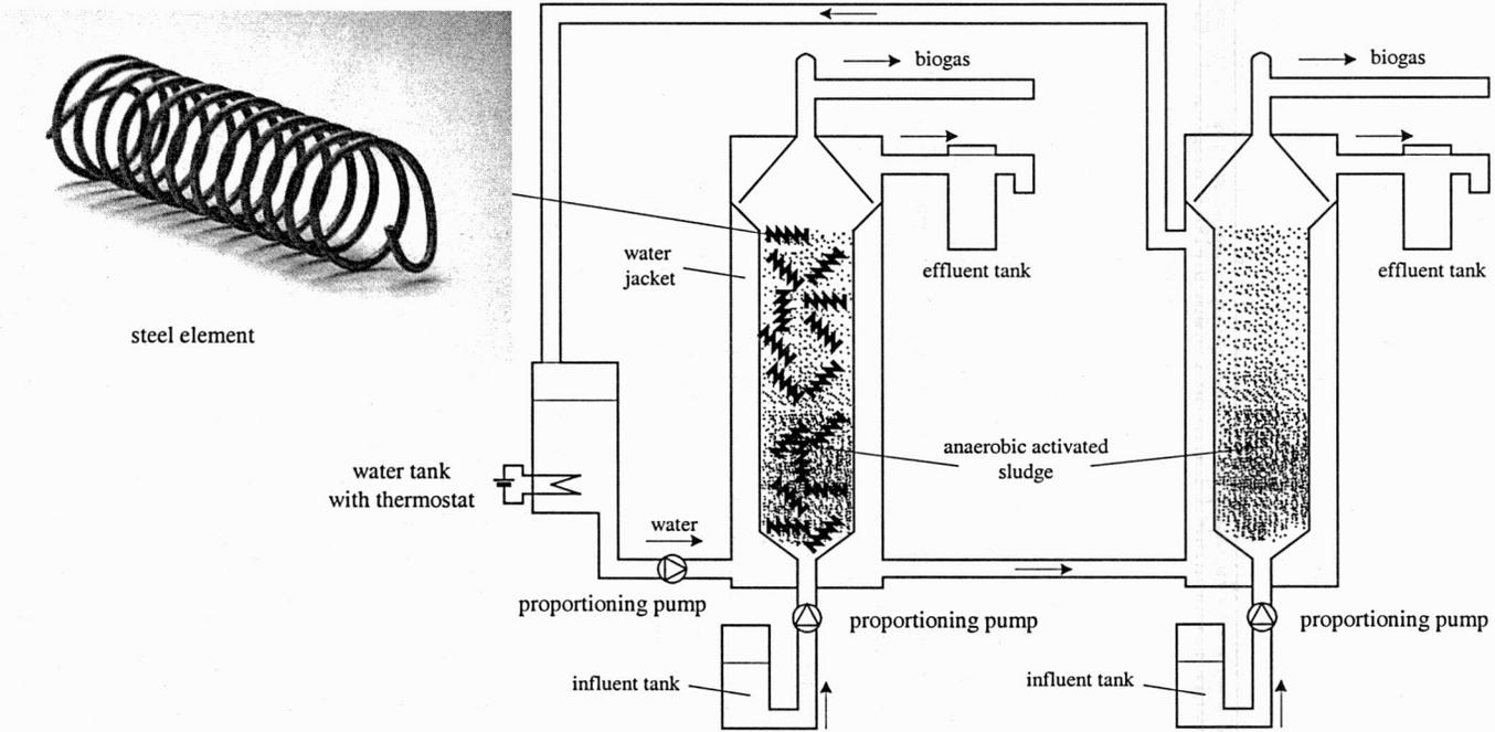
Fig. 1. Scheme of the installation
