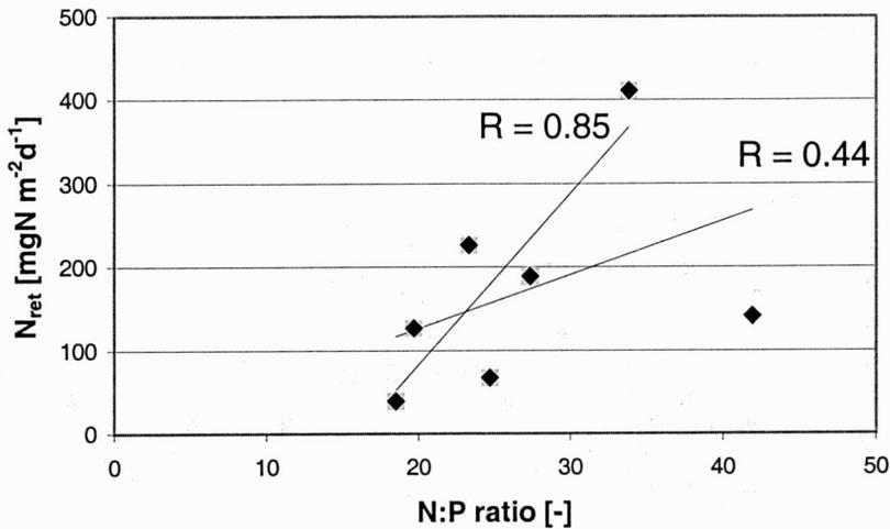
Fig. 3. Nitrogen retention versus N:P ratio in the Solina reservoir
