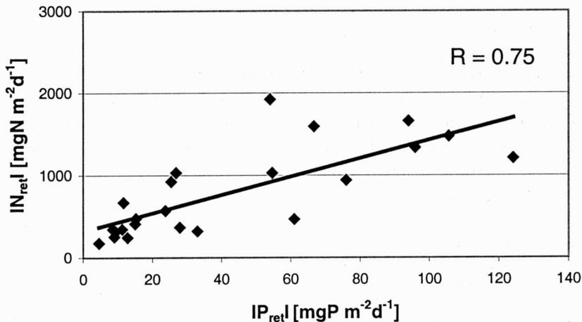
Fig. 4. The modulus of nitrogen retention versus the modulus of phosphorus retention in the Solina reservoir
