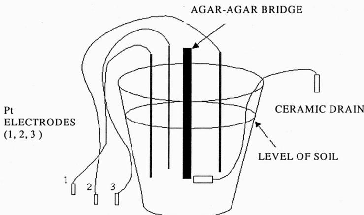
Fig. 1. Scheme of the test system
