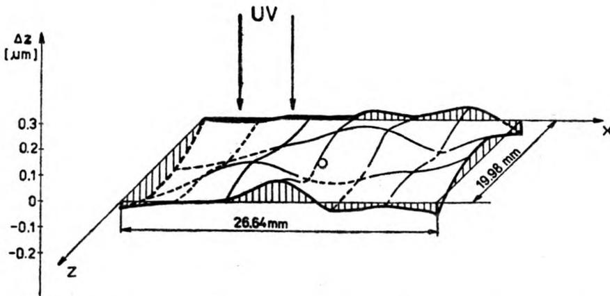
Fig. 11. Changes of the linear dimensions of the sample in the direction of irradiation
