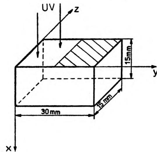
Fig. 1. Orientation of sample during irradiation
