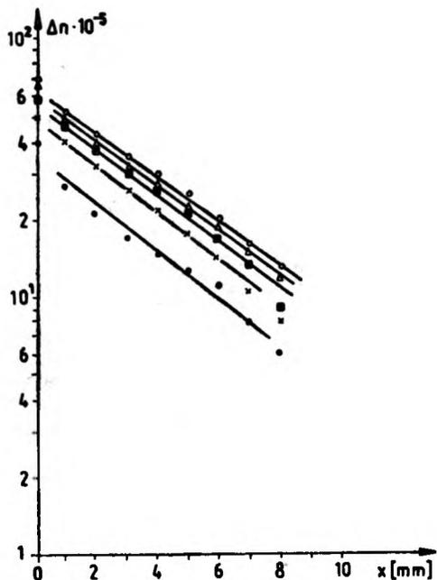
Fig. 5. Dependence of the changes of refractive index on the distance from the irradiated surface
