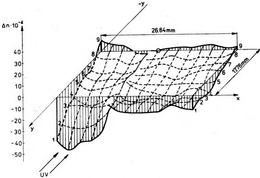
Fig. 8. Changes of refractive index in the  $x, y$  plane averaged along the sample thickness in the  $z$ -axis direction. Viewing direction perpendicular to that of irradiation. The numbers denote the successive scanning lines
