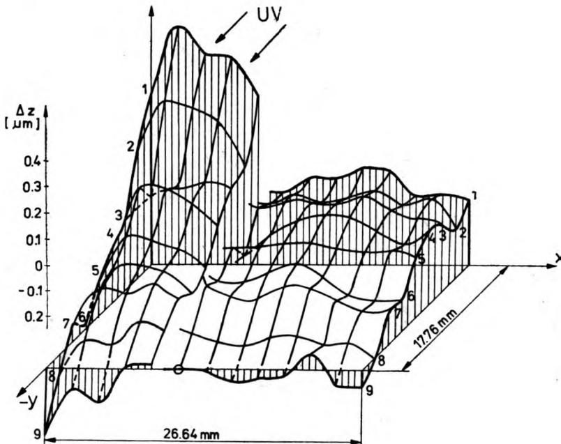
Fig. 9. Distribution of the thickness changes in the sample in the  $x, y$  plane. Viewing direction perpendicular to irradiation. The numbers denote successive scanning lines
