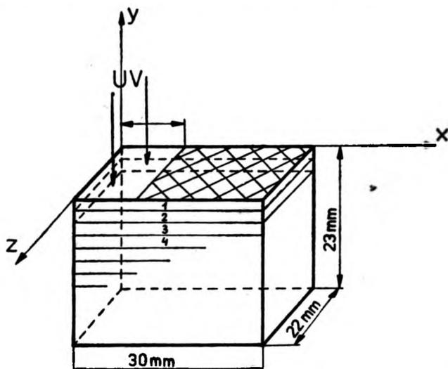
Fig. 6. Orientation of the sample during irradiation
