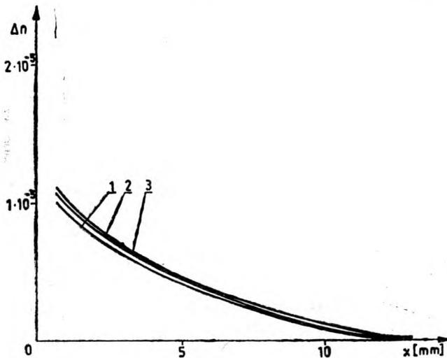
Fig. 2. Dependence of the changes of refractive index on the penetration depth of UV radiation for different exposure times: 1 - 20 min., 2 - 40 min., 3 - 60 min. During the irradiation the sample was kept at the 300 °C, the 400 Watt illuminating lamp was used
