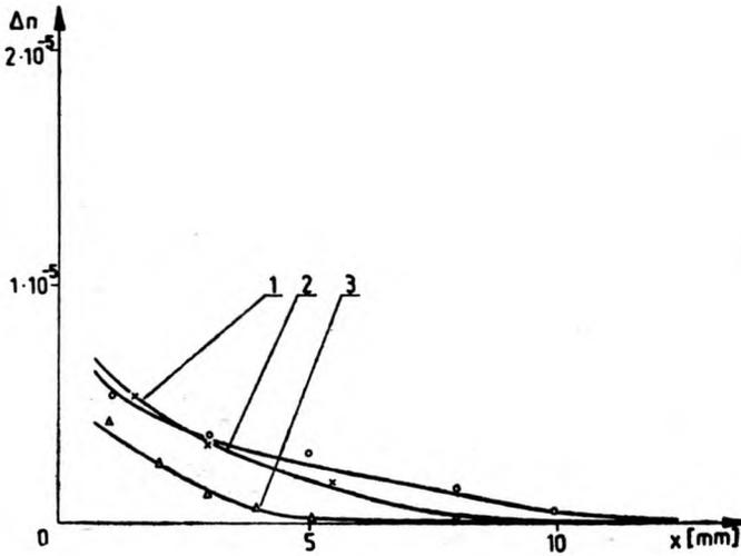
Fig. 3. Dependence of the changes of refractive index on the UV penetration depth for different kind of illumination lamps: 1 – 400 Watt illuminating lamp, 2 – HBO-200 lamp of Carl Zeiss (Jena), 3 – quartz lamp of L6/58 Helios type. During the irradiation the sample was kept at the 25 °C, exposure time – 1 h
