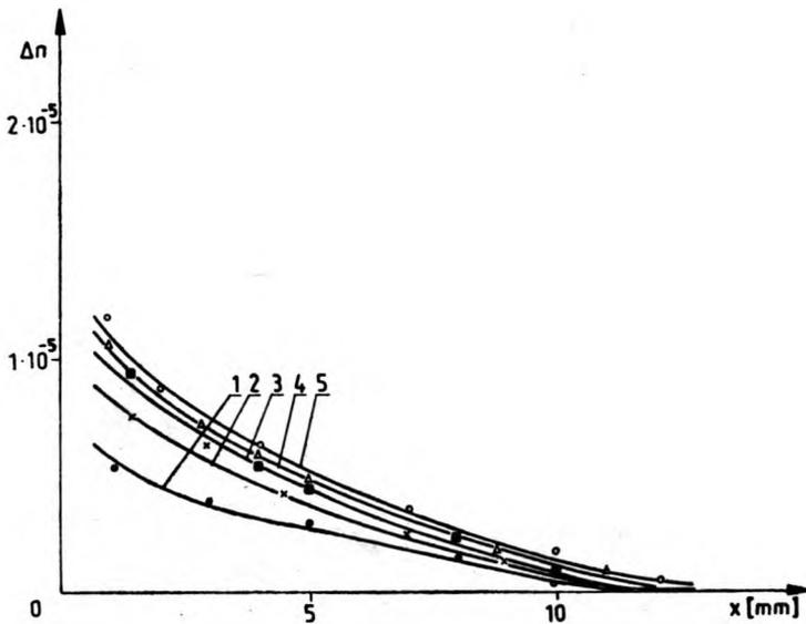
Fig. 4. Dependence of the changes of refractive index on the penetration depth of UV radiation for different temperatures at which the sample was kept during irradiation: 1 – 25 °C, 2 – 50 °C, 3 – 100 °C, 4 – 160 °C, 5 – 210 °C. Exposure time – 1 h, the illuminating 400 Watt lamp was used
