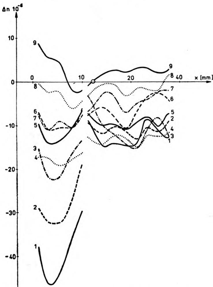
Fig. 7. Change of refractive index averaged along the total sample thickness for the successive scanning lines. The viewing direction perpendicular to that of irradiation
