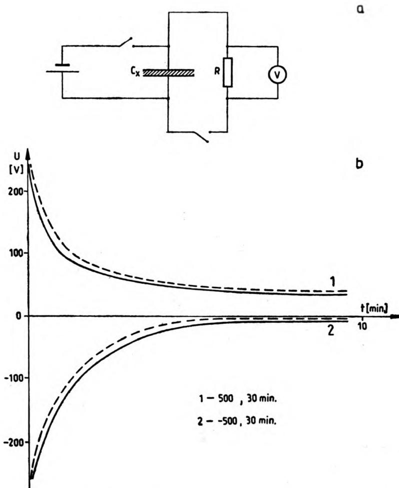
Fig. 2. Determination of the relaxation curves: a — measuring set-up, b — relaxation curves describing the irradiated (continuous line) and nonirradiated (broken line) parts ( $C_x$  — investigated sample,  $R$  — resistor,  $V$  — voltmeter)
