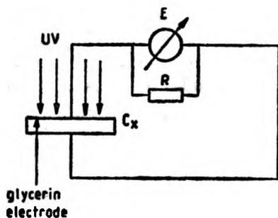
Fig. 3. Measuring setup for current flow ( $C_x$  — investigated sample,  $E$  — electrometer,  $R$  — resistor)
