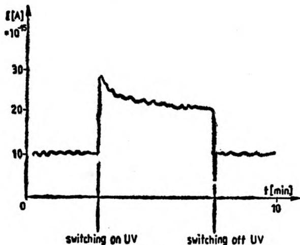
Fig. 4. Current flow observed in the glass sample during the irradiation by UV radiation
