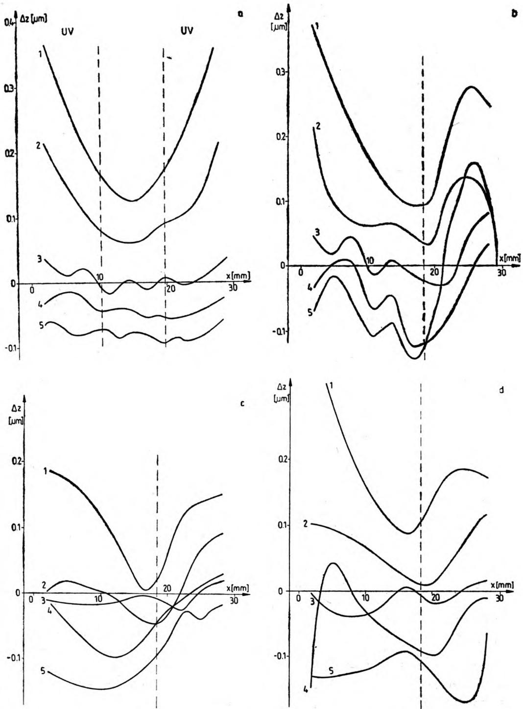
Fig. 9. Changes of the linear sizes of the glass sample after irradiation and application of the steady electric field. The numbers denote the successive scanning lines: a – after irradiation without the applied field, b – after application of the +12 kV voltage during 1 h, c – after application of the -12 kV voltage during 1 h, d – permanent changes
