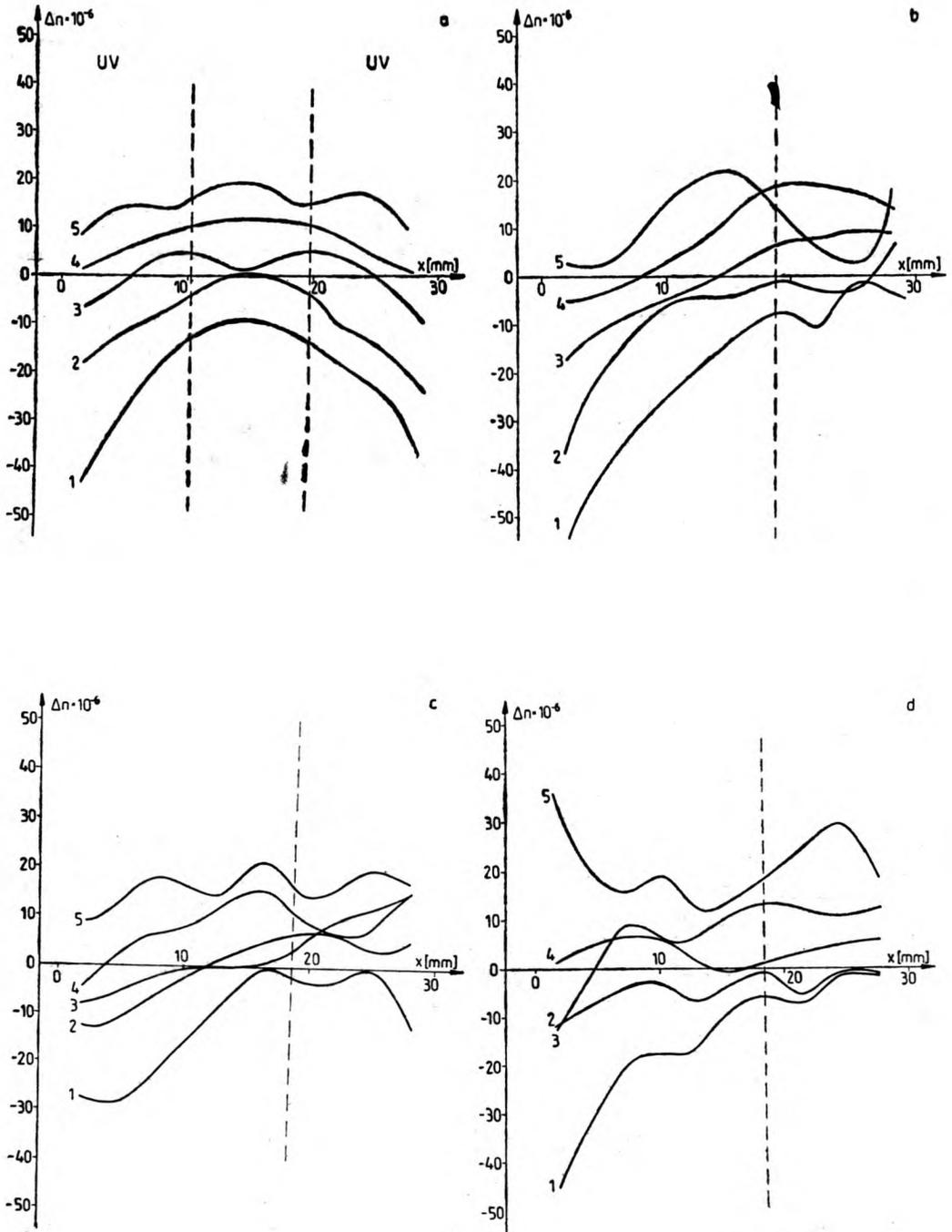
**Fig. 8.** Changes of refractive index in the glass sample after its irradiation and application of the steady electric field. The numbers denote the successive scanning lines: **a** — after irradiation without applied field, **b** — after application of the +12 kV voltage during 1 h, **c** — after application of the -12 kV voltage during 1 h, **d** — permanent change
