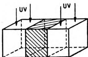
Fig. 6. Sample orientation during the irradiation
