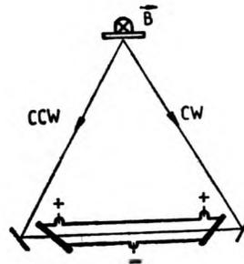
Fig. 3. Principle scheme of magnetic mirror laser gyro
