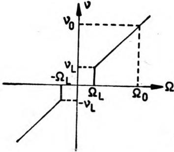
Fig. 1. Principle curve and lock-in region in laser gyro
