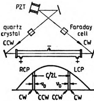
Fig. 2. Principle scheme of four-mode laser gyro
