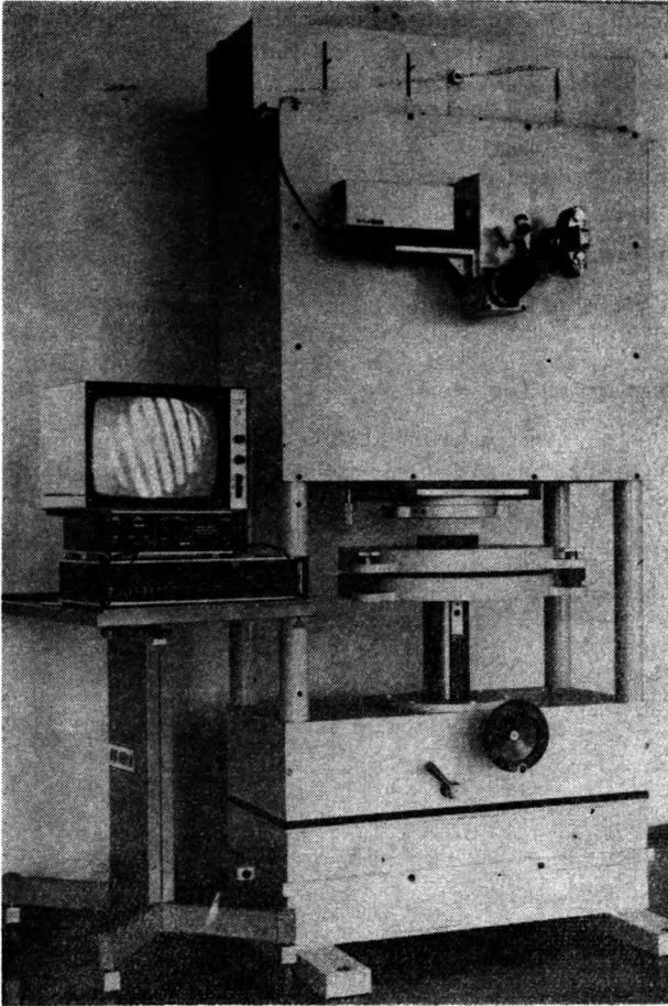
General view of the interferometer with the special electronic equipment to display interferometric fringes
