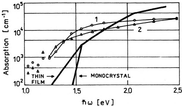
Fig. 2. Absorption coefficient spectra for: 1 – the deposited zinc phosphide layer, 2 – zinc phosphide layer after baking
