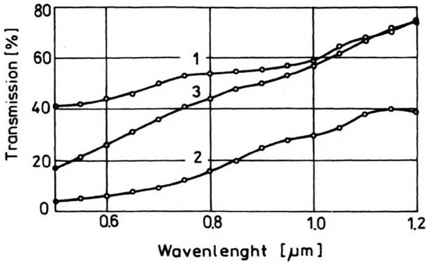
Fig. 1. Light transmission spectra for: 1 – porous glass without cover, 2 – porous glass with deposited zinc phosphide layer, 3 – porous glass with zinc phosphide after baking in 950 K in argon atmosphere
