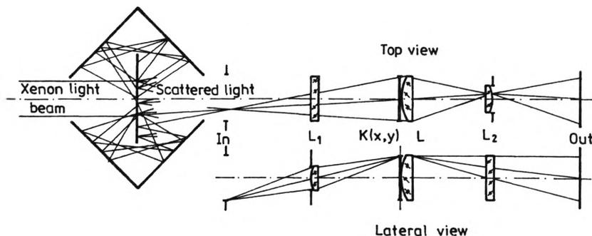
Fig. 1. Schematic representation of a non-coherent realizing an integral information.  $L_1$  and  $L_2$  - cylindrical lenses,  $K(x,y)$  - filter realizing transform kernel,  $L$  - spherical lens
