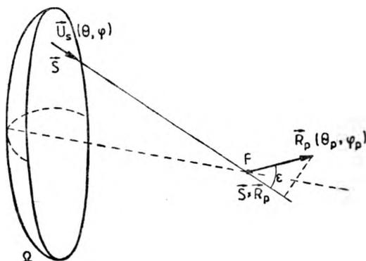
Fig. 1. Wolf transformation of the field  $U_s$ , given on the sphere  $\Omega$  into the field  $E$
