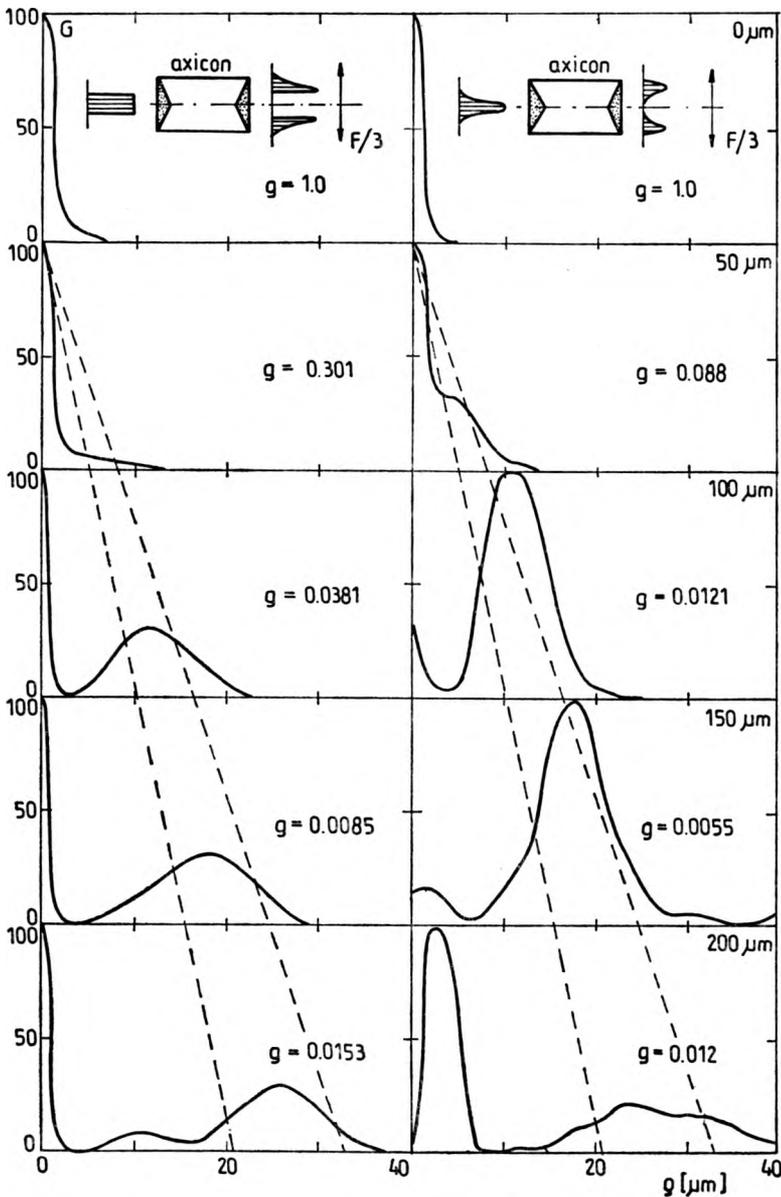
Fig. 6. Distributions of the relative power density  $G$  in the cross-sections distant by 50  $\mu\text{m}$  from one another, starting from the focus vs. the distance from the optical axis: left hand column - rectangular beam, right hand column - Gaussian beam ( $g$  - ratio of the maximal power density at given cross-section to the maximal power density at the focus)
