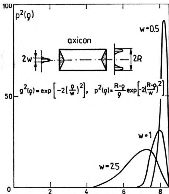
Fig. 4. Transformation of the power density in a Gaussian beam by an axicon ( $w$  - beam radius,  $\varrho$  - distance from the optical axis,  $R$  - radius of the axicon)
