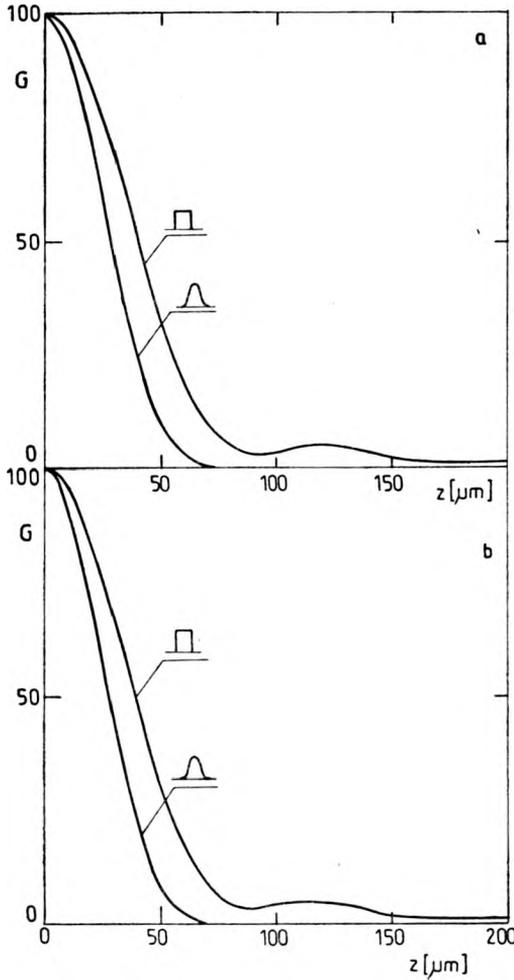
Fig. 5. Distributions of relative power density  $G$  as a function of the distance  $z$  from the focus, calculated along the optical axis for both the Gaussian and rectangular beams: a – according to the rigorous formula, b – according to the Wolf transformation
