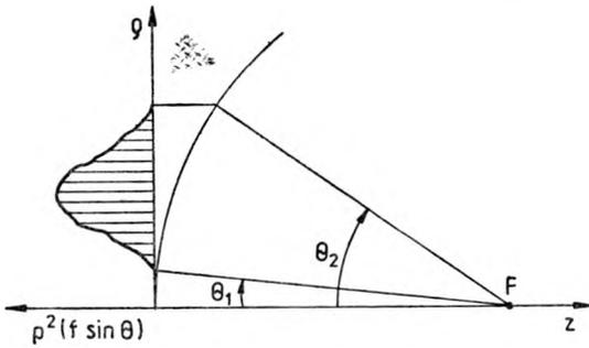
Fig. 2. Wolf transformation of the power density in the entrance beam by an ideal optical system
