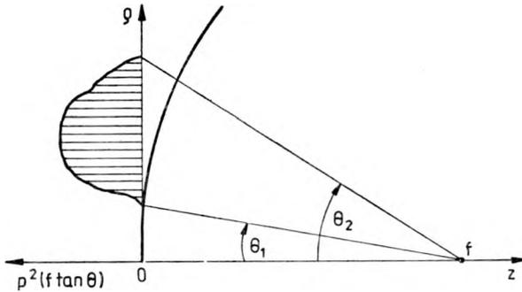
Fig. 3. Transformation of the power density in the entrance beam by an ideal optical system according to formula (7)
