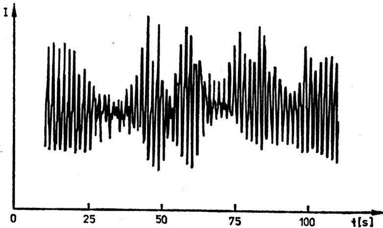
Fig. 4. Time dependent intensity variation of the far-field diffraction pattern at the applied voltage of 11 V
