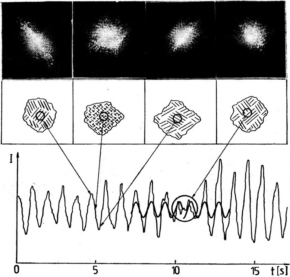
Fig. 3. Diffraction at a single domain of the "seesaw oscillation". Applied voltage  $U = 11$  V
