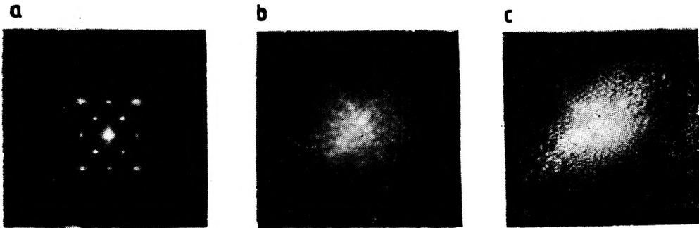
Fig. 2. Fourier spectrum of the sample (a), far-field diffraction patterns at the beam width of 300  $\mu\text{m}$  (b) and 8  $\mu\text{m}$  (c). Applied voltage  $U = 11 \text{ V}$
