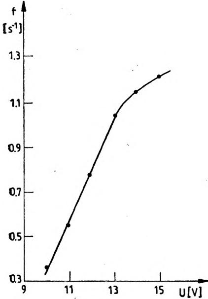
Fig. 5. Dependence of the frequency of the "seesaw oscillation" on the applied voltage
