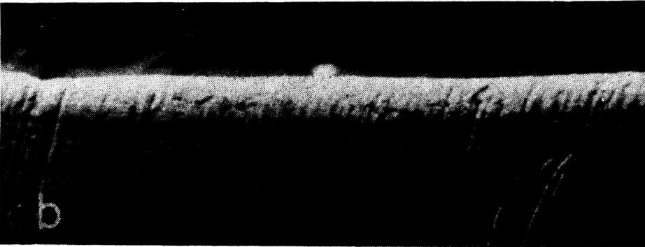
Fig. 1. Photos of the metallographic cross-sections of two irradiated regions of the sample. The photo **a** was made with the aid of the Eptyp 2 microscope, and **b** — by using the BS 300 microscope. Maximal thickness of the hardened layer amounts to 80 and 100  $\mu\text{m}$ , respectively
