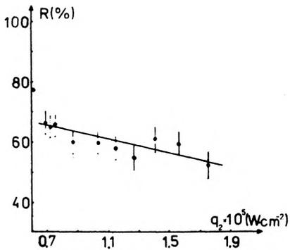
Fig. 2. Dependence of the reflection coefficient  $R$  upon the power density  $Q_2$  of the incident beam
