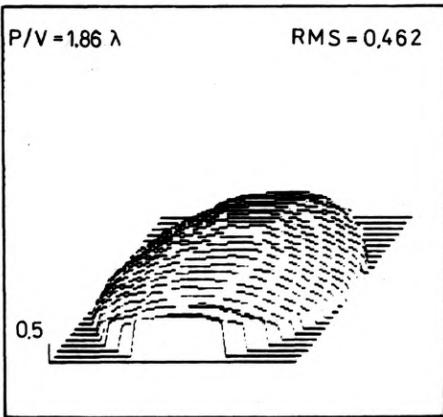
Fig. 3. Example of 2-D phase distribution decoded from a fringe pattern bounded with circular aperture
