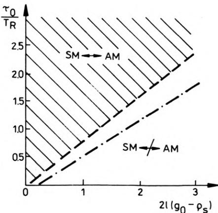
Fig. 5. Applicability limits for AM, for admissible value of error 10% (---), and 20% (-.-.-)
