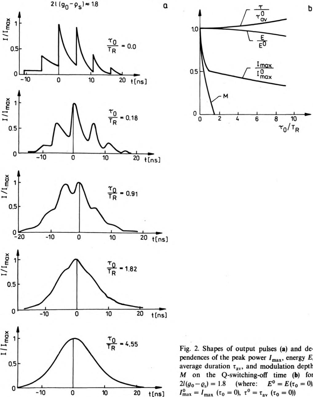
Fig. 2. Shapes of output pulses (a) and dependences of the peak power  $I_{max}$ , energy  $E$ , average duration  $\tau_{av}$ , and modulation depth  $M$  on the Q-switching-off time (b) for  $2l(g_0 - \rho_s) = 1.8$  (where:  $E^0 = E(\tau_0 = 0)$ ,  $I_{max}^0 = I_{max}(\tau_0 = 0)$ ,  $\tau^0 = \tau_{av}(\tau_0 = 0)$ )
