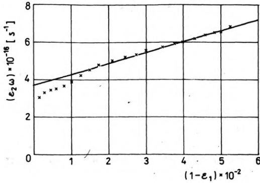
Fig. 2. Dependence of  $\epsilon_2$  on  $1 - \epsilon_1$  for the chromium layers evaporated in the temperature  $T_s = 200^\circ C$
