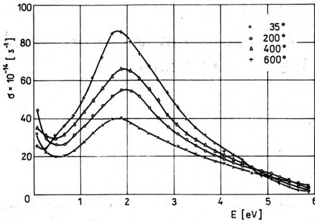
Fig. 1. Spectral dependence of the optical conductivity  $\sigma$  for the chromium layers evaporated at the rate  $v \sim 20 \text{ \AA/s}$  onto the heated substrate of different temperatures
