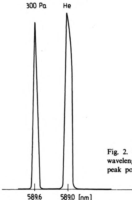
Fig. 2. Current pulses amplitude (a.u.) as a function of the laser wavelength for sodium vapour density  $10^{19} \text{ m}^{-3}$  and the laser pulse peak power 400 W
