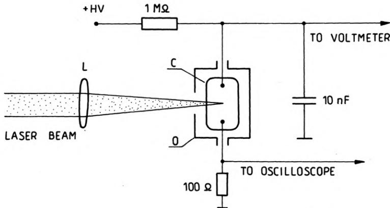
Fig. 1. Experimental setup. O – oven, C – pyrex cell, L – lens
