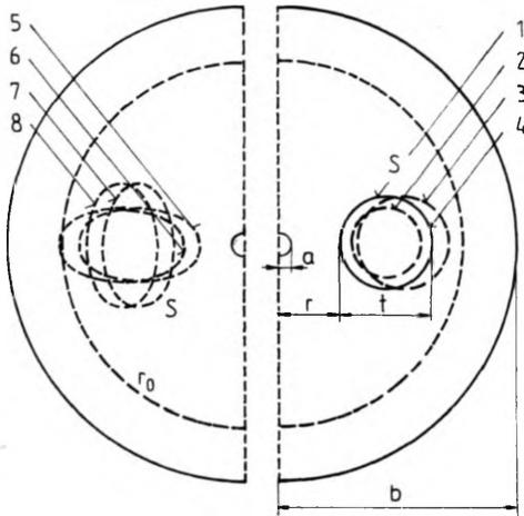
Fig. 1. Circular and elliptical deformation of stress-applying parts of a Panda fibre.  $S$  – stress-applying parts. 1 – basic structure, 2 – diminished diameter of stress-applying parts, 3 – horizontal translation, 4 – basic structure without a fibre core  $\alpha_{cr} = \alpha_{cl}$ , 5 – horizontal elliptical deformation, 6 – translated horizontal deformation, 7 – vertical deformation, 8 – translated vertical deformation
