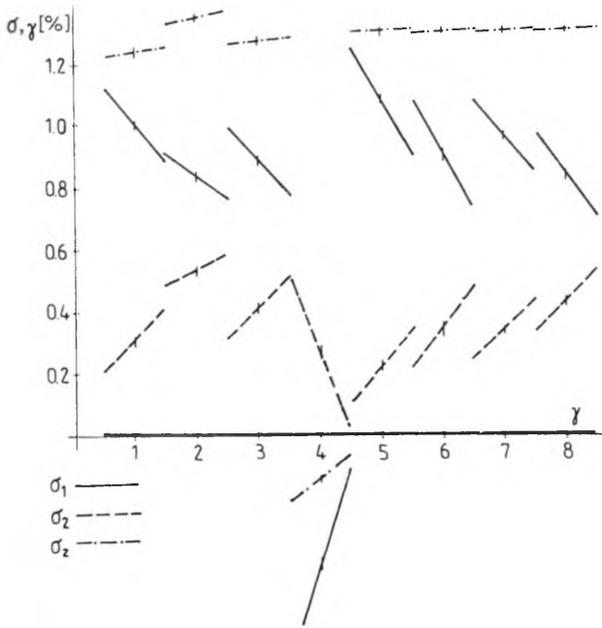
Fig. 3. Mechanical stresses in a fibre core:  $\sigma_1, \sigma_2$  – principal stresses in horizontal and vertical directions, respectively;  $\sigma_z$  – axial stress,  $\gamma$  – rotation angle
