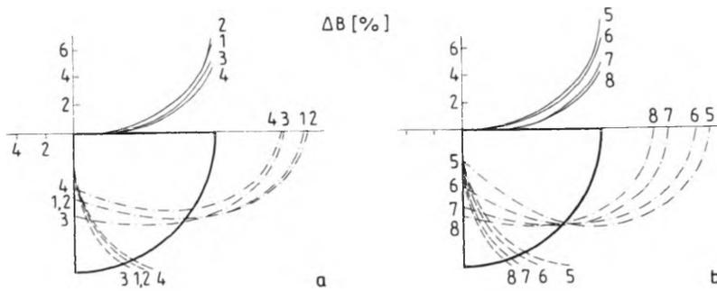
Fig. 4. Deviations of birefringence in a fibre core: a – horizontal axis, b – vertical axis
