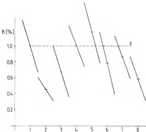
Fig. 2. Birefringence of Panda fibre structures shown in Fig. 1
