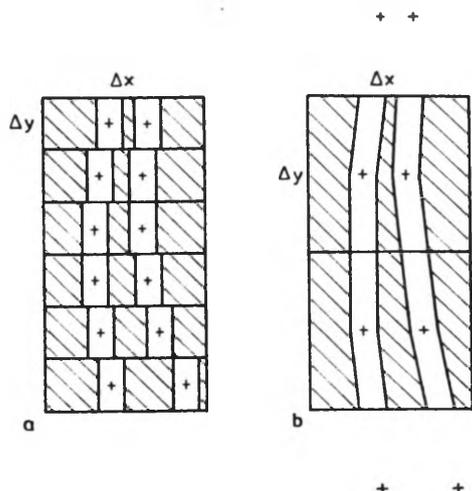
Fig. 2. Ways of cell-connecting: **a** — decrease of cell height and increase of number of cells, **b** — “plotter interpolation”
