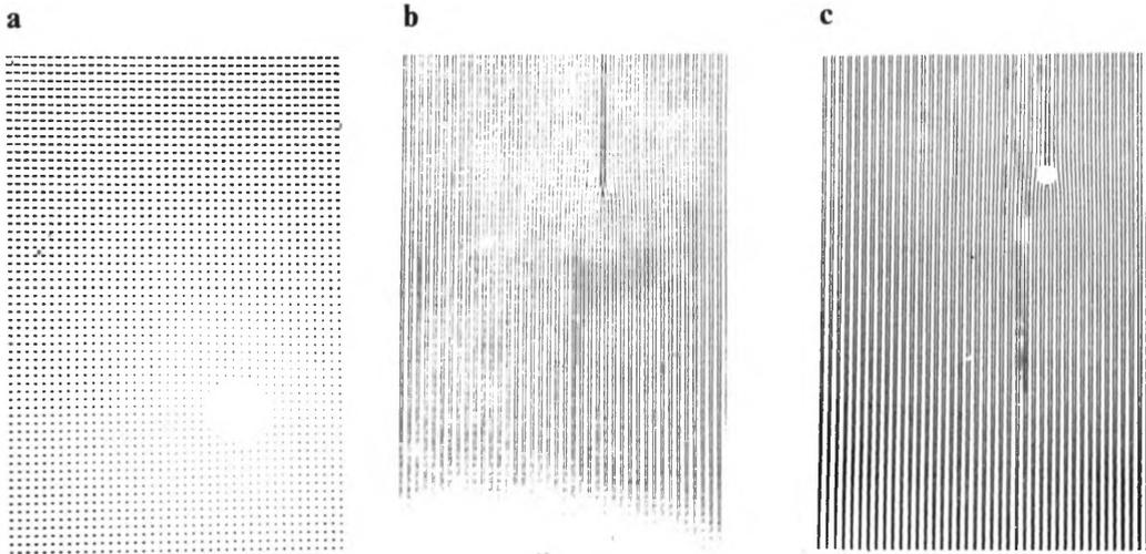
Fig. 5. Filters' maps: **a** – classical Lohmann method, **b** – two-aperture Lohmann method with cell connecting, **c** – as above with intercepted centre
