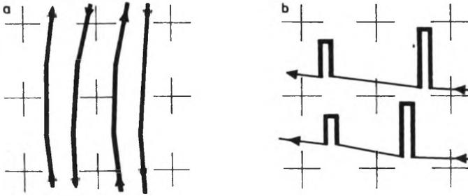
Fig. 4. Ways of pen up (thin line) and down (thick line) in producing hologram encoded by: **a** – two-aperture Lohmann method with cell-connecting, **b** – classical Lohmann method
