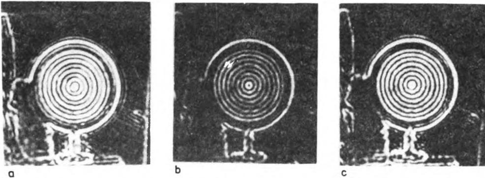
Fig. 8. True output images when using filters encoded by: **a** — classical Lohmann method, **b** — two-aperture Lohmann method with cell-connecting, **c** — as above with intercepted centre
