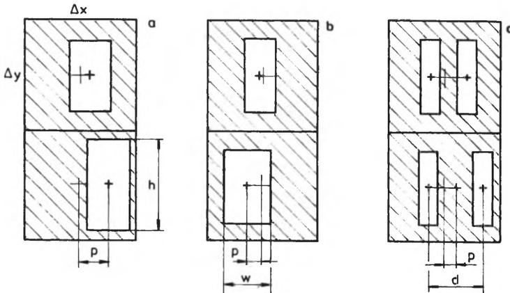
Fig. 1. Lohmann's detour phase methods of CGH encoding: **a** –  $h = (A/A_{\max})\Delta x$ ,  $p = (\text{phase}/2\pi)\Delta y$  (classical Lohmann method), **b** –  $w = \sin[(A/A_{\max})(\pi/2)]\Delta y/2$ ,  $p = (\text{phase}/2\pi)\Delta y$ , **c** –  $d = \cos[(A/A_{\max}) \times (\pi/2)]\Delta y/2$ ,  $p = (\text{phase}/2\pi)\Delta y$  (two-aperture Lohmann method)
