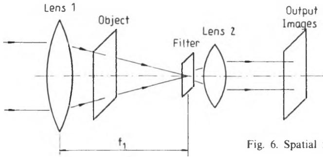
Fig. 6. Spatial filtering system used in experiments
