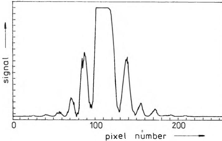
Fig. 3. Fraunhofer's diffraction on circular aperture
