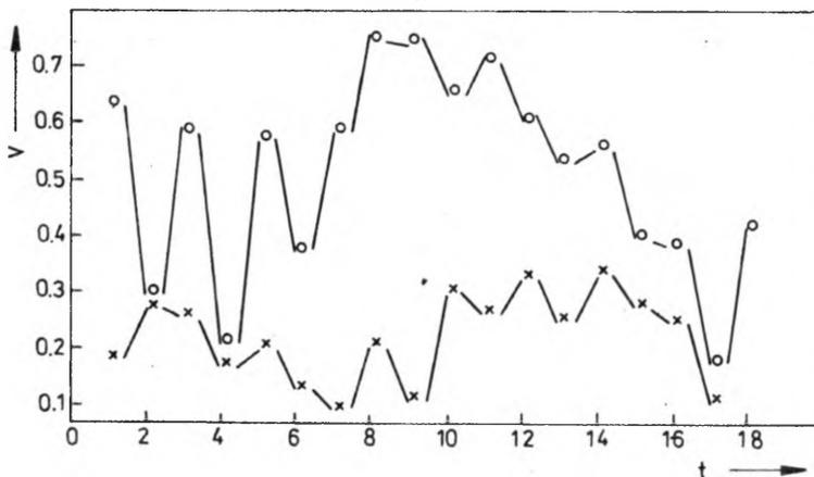
Fig. 7. Contrast ( $V$ ) time change of interferograms in Michelson's interferometer in 18 consecutive recordings (one recording takes 48 milliseconds) at  $\Delta l = 2$  cm (o) and  $\Delta l = 46$  cm (+)
