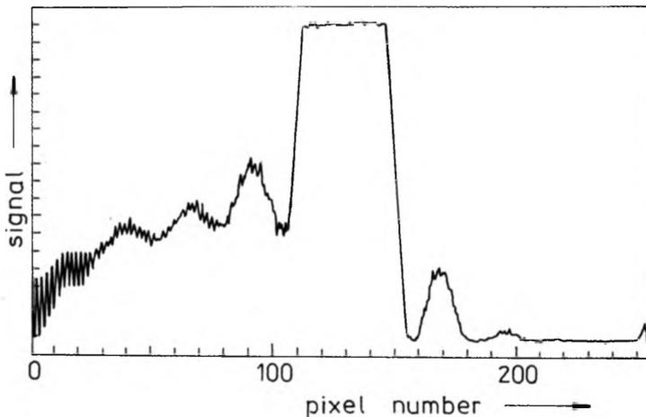
Fig. 5. Fraunhofer's diffraction by the slit at significantly supersaturated zero maximum
