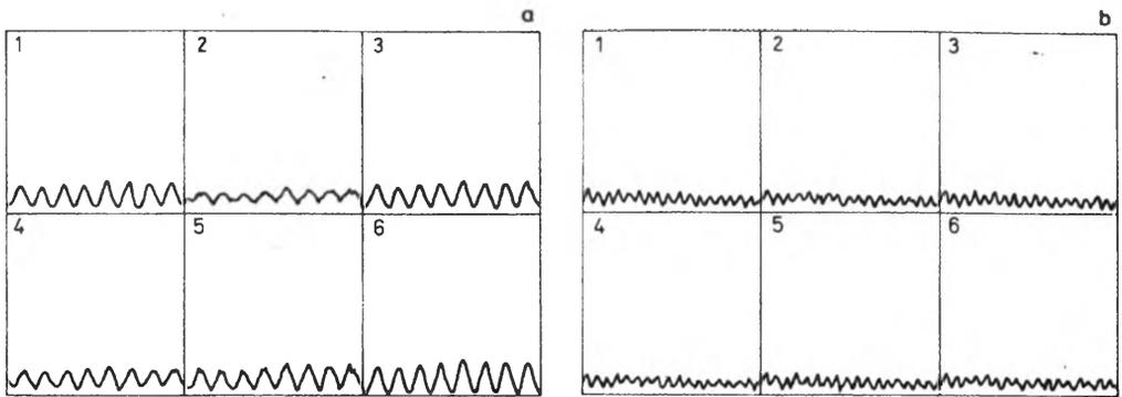
Fig. 6. Interference fringes in Michelson's interferometer at a path difference of:  $\Delta l = 2$  cm (a) and  $\Delta l = 46$  cm (b). Depicted are 6 recordings
