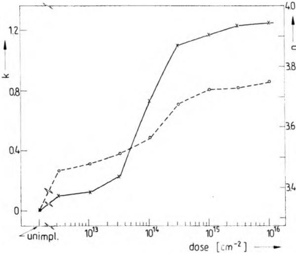
Fig. 3. Optical constants  $n$  (solid line) and  $k$  (dashed line) of GaP samples implanted with 100 keV  $\text{Ar}^+$  ions as a function of a dose ( $\lambda = 632.8$  nm)
