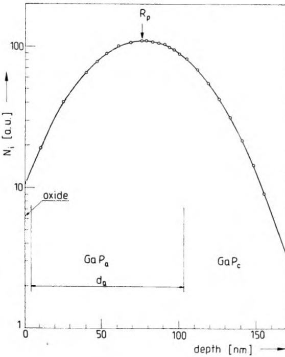
Fig. 5. Thickness of disordered layer  $d_a$  in comparison with distribution of implanted ions ( $\text{Ar}^+$   $10^{16} \text{cm}^{-2}$ , 100 keV) vs the depth
