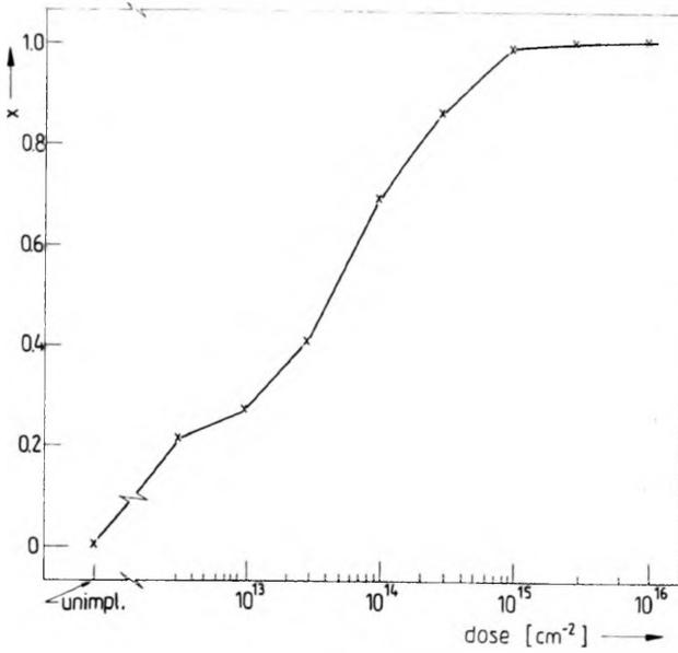
Fig. 4. Degree of amorphousness vs a dose of 100 keV  $\text{Ar}^+$  ions implanted to GaP
