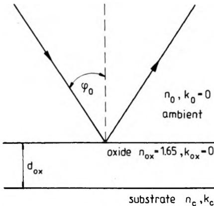
Fig. 1. Three-phase model of unimplanted GaP
