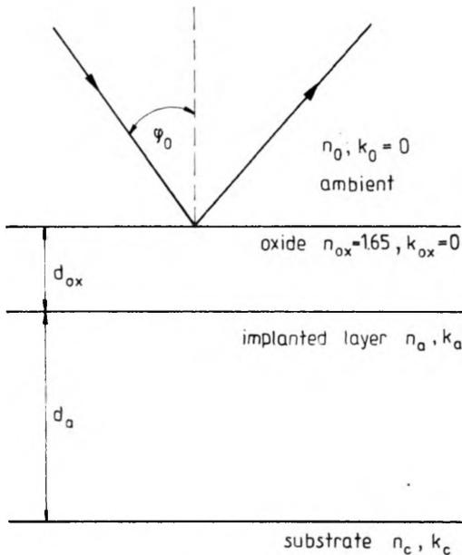
Fig. 2. Four-phase model of implanted GaP
