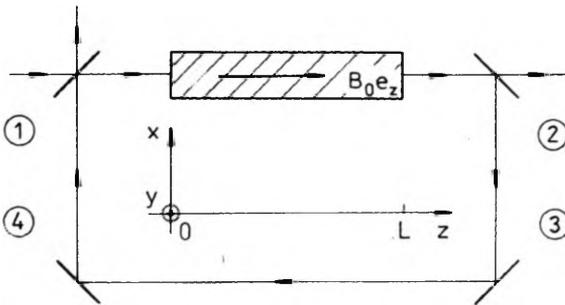
Fig. 1. Nonlinear ring resonator (1-4 mirrors)
