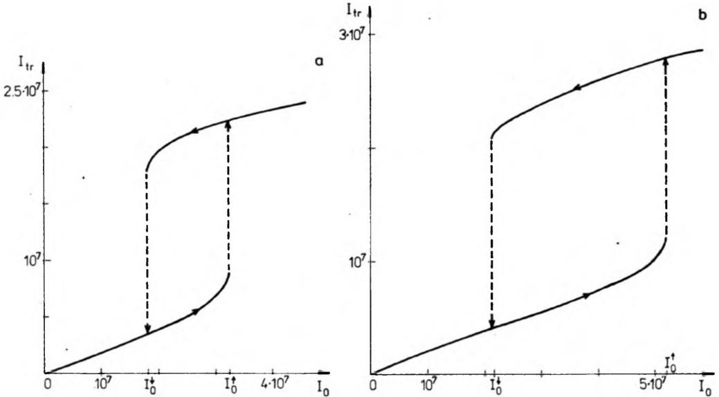
Fig. 2. Intensity bistability in the ring resonator referring to the phase increases:  $\Phi_{\perp} = \Phi_{\parallel} = \pi/6$  (a), and  $\Phi_{\perp} = \pi/3$ ,  $\Phi_{\parallel} = \pi/2$  (b)
