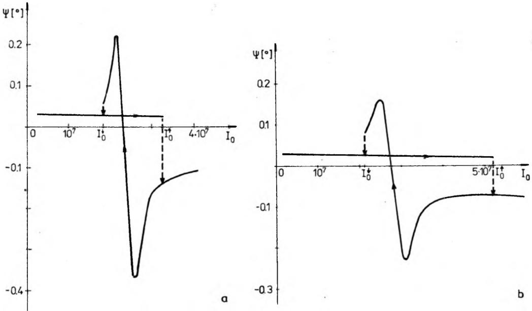
Fig. 4. Bistability of the orientation angle of the polarization ellipse referring to the phase increases:  $\Phi_{\perp} = \Phi_{\parallel} = \pi/6$  (a),  $\Phi_{\perp} = \pi/3$ ,  $\Phi_{\parallel} = \pi/2$  (b)
