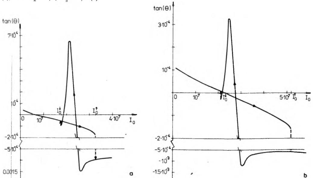
Fig. 3. Bistability of the ratio of the polarization ellipse semiaxes referring to the phase increases:  $\Phi_{\perp} = \Phi_{\parallel} = \pi/6$  (a),  $\Phi_{\perp} = \pi/3$ ,  $\Phi_{\parallel} = \pi/2$  (b)
