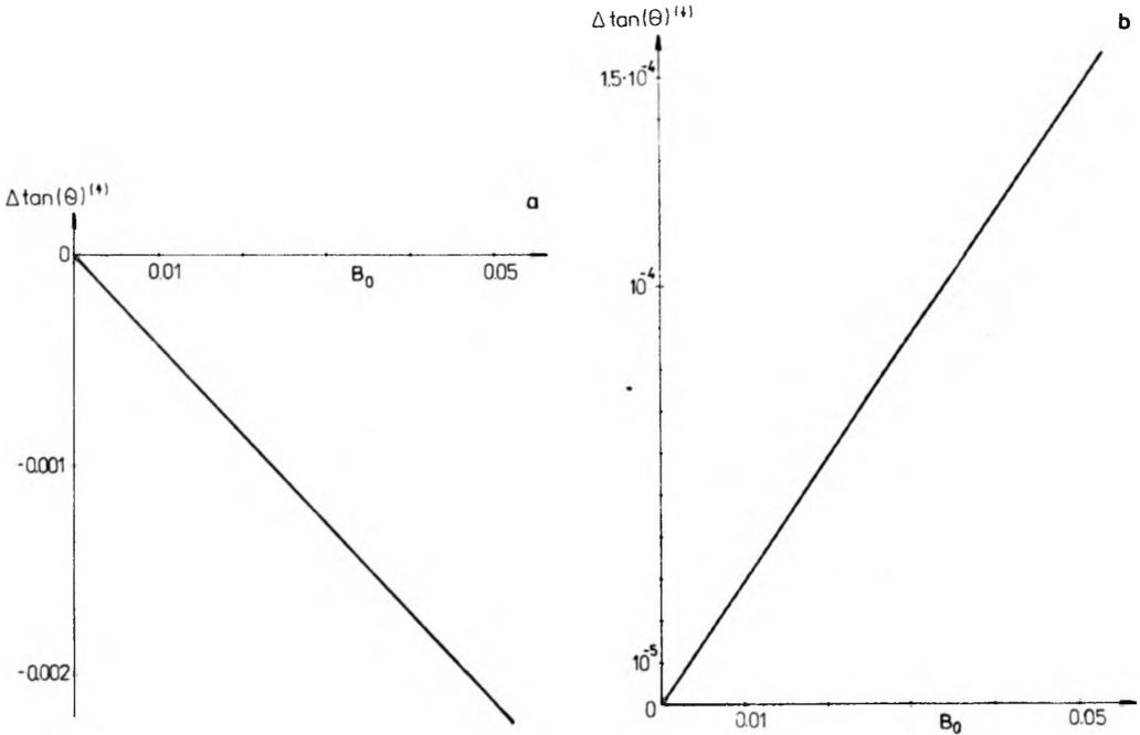
Fig. 7. Heights of the nonlinear "jumps" of the ratio of the polarization ellipse semi-axes of the transmitted light as functions of the external magnetic field referring to the incident light intensities: **a** -  $I_0 = I_0^{\downarrow}$ , **b** -  $I_0 = I_0^{\uparrow}$
