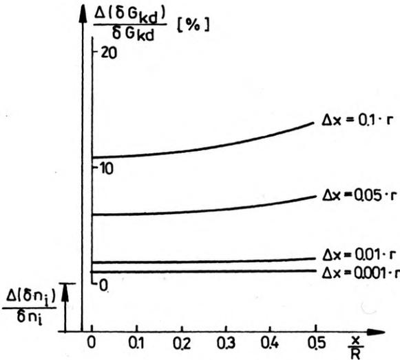
Fig. 7. Relative error of the correcting wavefront for real run of the ray through the examined object
