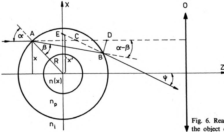
Fig. 6. Real run of the ray through the object examined
