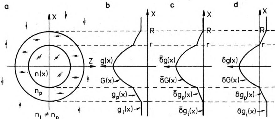
Fig. 2. Wavefront after its passage through the object examined ( $n_i \neq n_p$ ): **a** – object, **b** – wavefront, **c** – wavefront referred to the object coat wavefront, **d** – wavefront referred to the immersion wavefront
