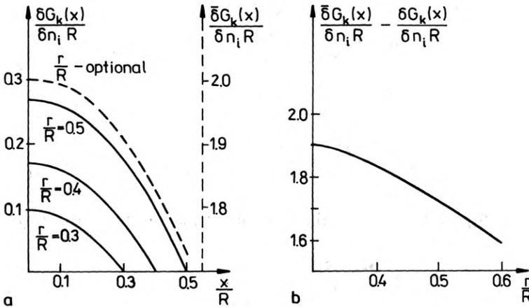
Fig. 3. Normalized correcting wavefronts (a) and the dependences among them (b)
