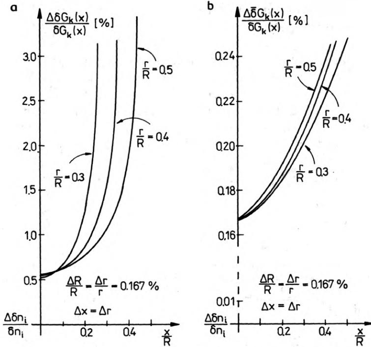
Fig. 4. Relative errors of the correcting wavefronts: a – for the wavefront  $\delta g(x)$ , b – for the wavefront  $\bar{\delta} g(x)$
