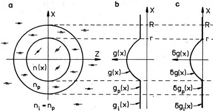
Fig. 1. Wavefront after its passage through the object examined ( $n_i = n_p$ ): a – object, b – wavefront, c – wavefront referred to the object coat wavefront
