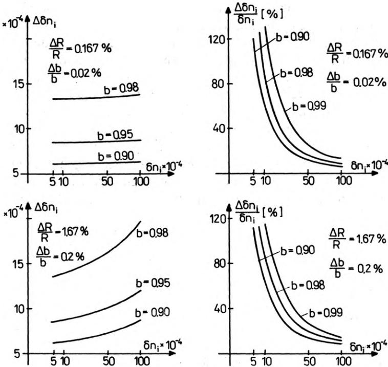
Fig. 7. Absolute and relative measurement errors of the refractive index difference  $\delta n_i$  for different accuracies of both the coat diameter measurement  $\Delta R/R$  and the radial shearing parameter  $\Delta b/b$ . Case of the light waveguide  $R = 6 \times 10^{-5}$
