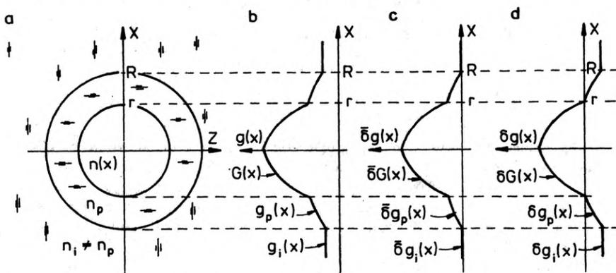
Fig. 1. Wavefronts after having passed the object under test: a - object, b - wavefront, c - wavefront referred to the immersion, d - wavefront referred to the clad
