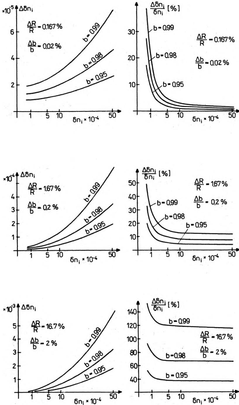
Fig. 5. Absolute and relative measurement errors for the refractive index difference for different accuracies of the coat diameter measurement  $\Delta R/R$  and different value of the radial shearing parameter  $\Delta b/b$ . Case of the preform  $R = 6 \times 10^{-3}$
