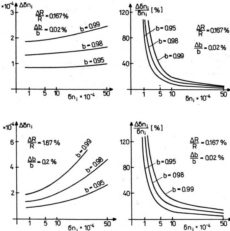
Fig. 6. Absolute and relative measurement errors of the refractive index difference for different accuracies of both the coat diameter measurement  $\Delta R/R$  and the radial shearing parameter  $\Delta b/b$ . Case of thick-core waveguide  $R = 6 \times 10^{-4}$  m
