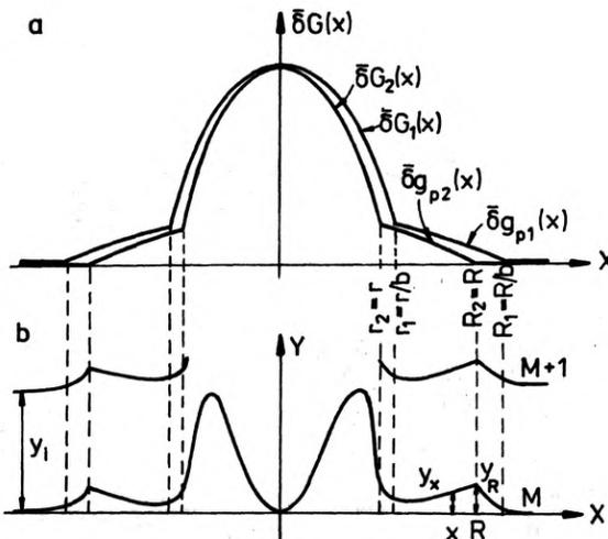
Fig. 2. Interfering wavefronts (a) and the result of interference of radial shearing type (b)
