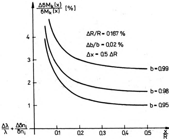
Fig. 8. Relative error of the functions correcting the interference order  $\delta M_k(x)$ : a - object, b - wavefront, c - wavefront referred to the immersion, d - wavefront referred to the clad
