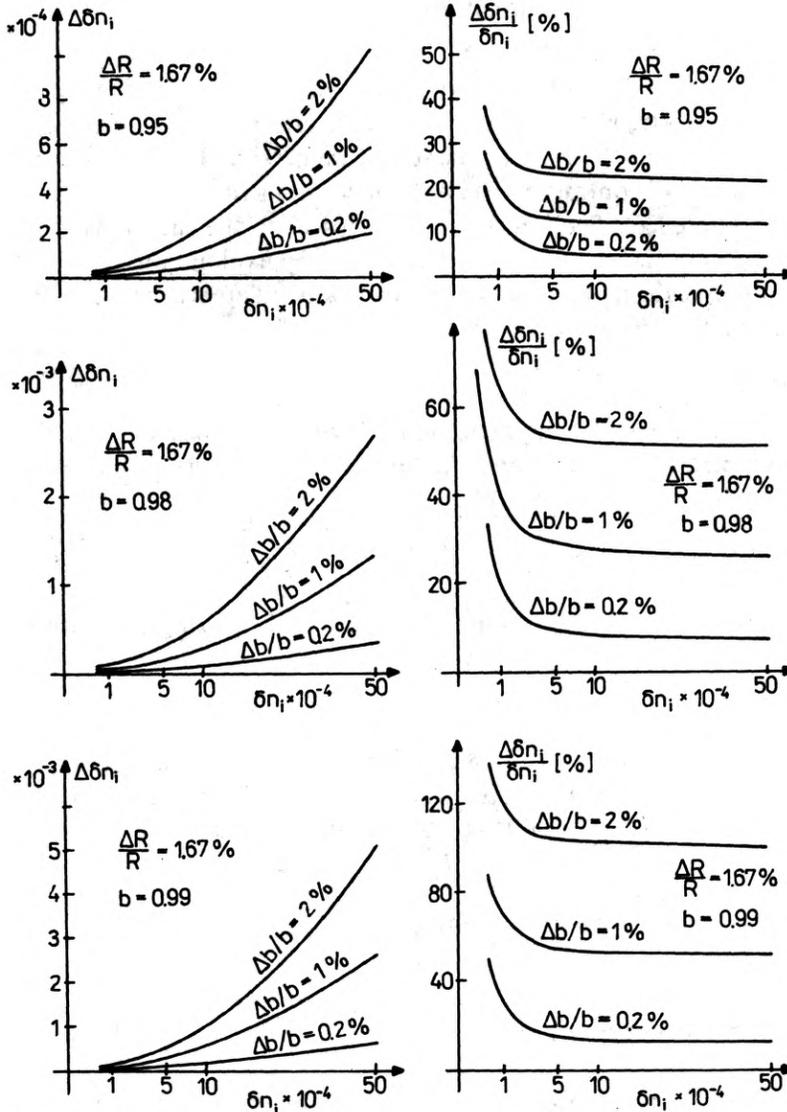
Fig. 4. Absolute and relative measurement errors for the refractive index difference  $\delta n_i$  for an established accuracy of the coat diameter measurement  $\Delta R/R = 1.67\%$ . Case of the preform  $R = 6 \times 10^{-3}$  m
