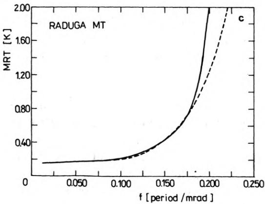
Fig. 2. Calculated and measured MRT for the reference systems: **a** - for AGA 780, **b** - for Rubin MT, **c** - for Raduga MT (— measured values, - - - calculated ones)
