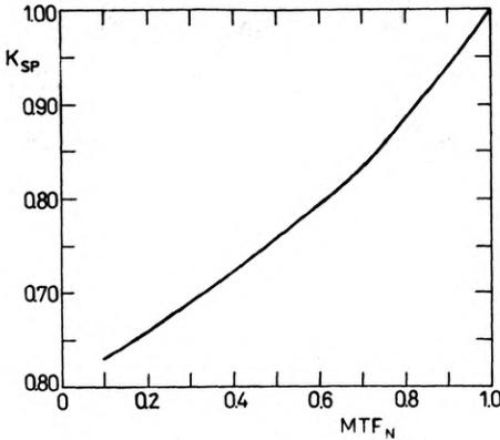
Fig. 1. Typical values of normalized noise equivalent bandwidth
