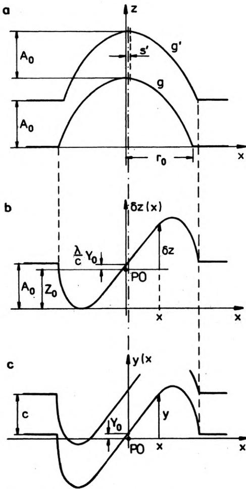
Fig. 6. Transversal shearing interference of: **a** – mutually interfering wavefronts  $g_1$  and  $g_2$ ; **b** – optical path difference  $\delta z$ ; **c** – interference fringes on the interferogram
