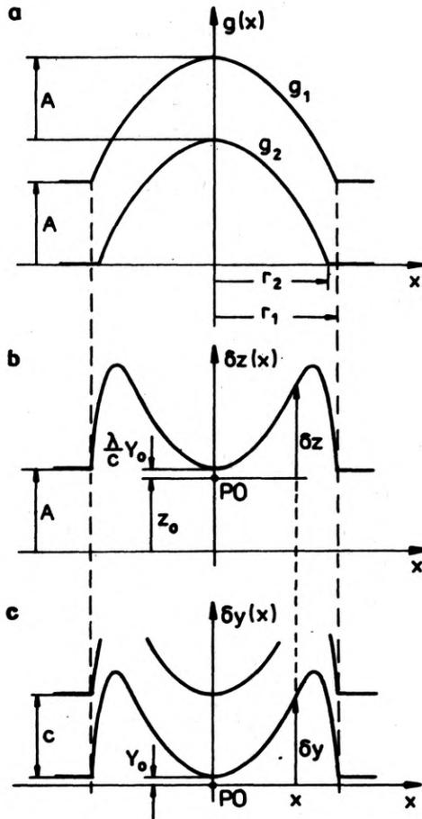
Fig. 1. Radial shearing interferometry: **a** – mutually interfering wavefronts  $g_1$  and  $g_2$ ; **b** – optical path difference  $\delta z$ ; **c** – interference fringes on the interferogram
