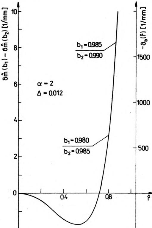
Fig. 5. Differences of normed orders of interference with different shearing parameters  $b$ . The derivative  $\partial_b(f)$  of the normed order of interference with respect to the parameter  $b$
