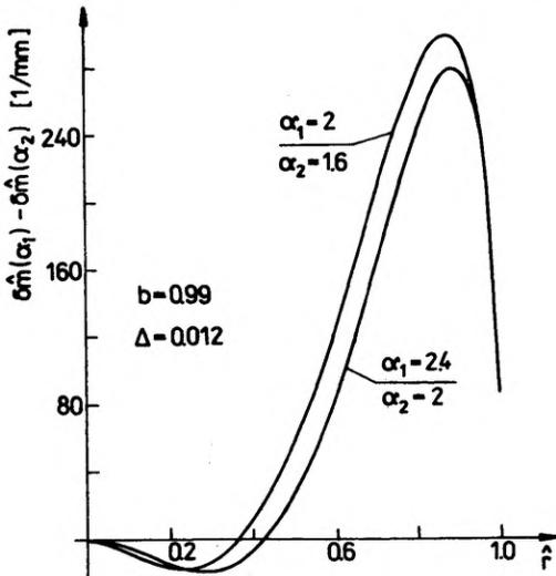
Fig. 3. Differences of normed orders of interference as depending on different values of  $\alpha$
