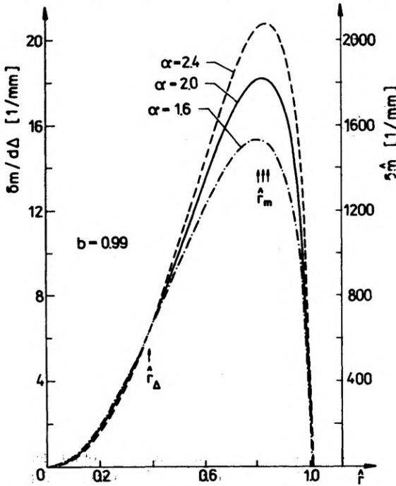
Fig. 2. Ratio of the relative order of interference  $\delta m$  to the product of the core diameter  $d$  and the parameter  $\Delta$  related to  $\alpha$ . Normed order of interference  $\delta \hat{m}$  depending on  $\alpha$
