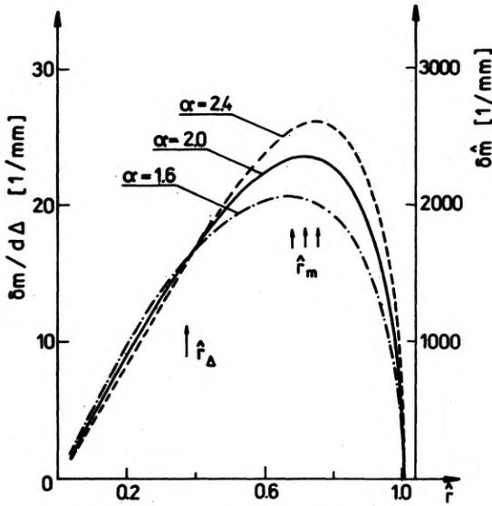
Fig. 7. Ratio of the relative order of interference  $\delta m$  to the product of the core diameter  $d$  and the parameter,  $\Delta$ . Normed order of interference  $\delta \hat{m}$  depending on  $\alpha$
