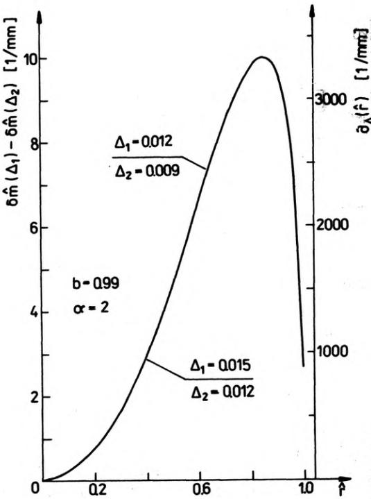
Fig. 4. Differences of normed orders of interference with different parameters  $\Delta$ . The derivative  $\partial_{\Delta}(f)$  of the normed order of interference with respect to the parameter  $\Delta$
