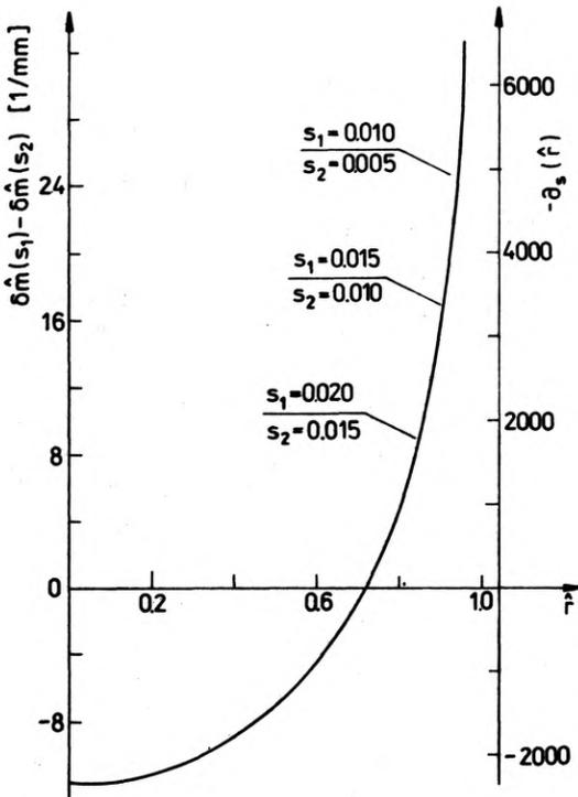
Fig. 10. Differences of normed orders of interference with different shearing parameters  $s$ . The derivative  $\partial_s(\hat{r})$  of the normed order of interference with respect to the shearing parameter  $s$
