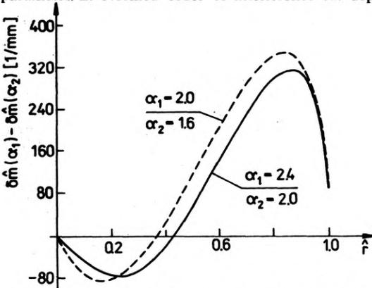
Fig. 8. Differences of the normed orders of interference as depending on different values of  $\alpha$
