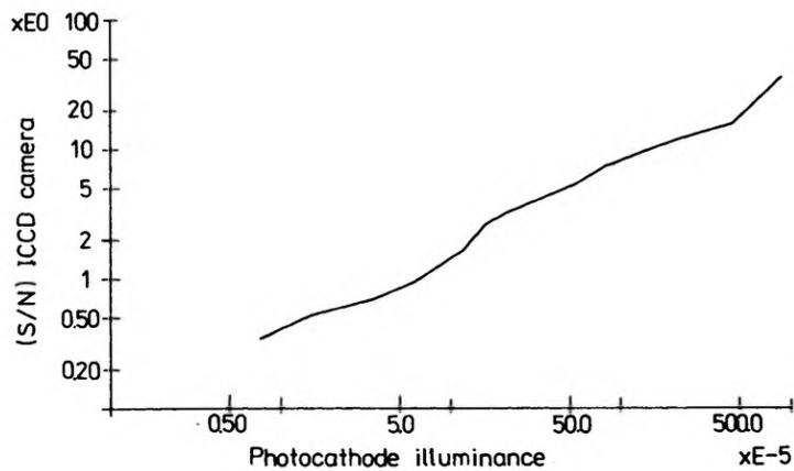
Fig. 8. S/N ratio for ICCD camera against photocathode illuminance
