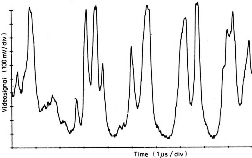
Fig. 3. Photon noise on digital oscilloscope display in the measurement of CICCD signal with 0.5 MHz test pattern
