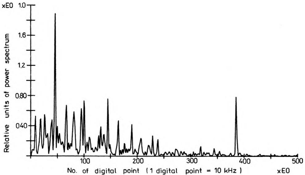
Fig. 13. Calculation of power spectrum of structural noise of CICCD
