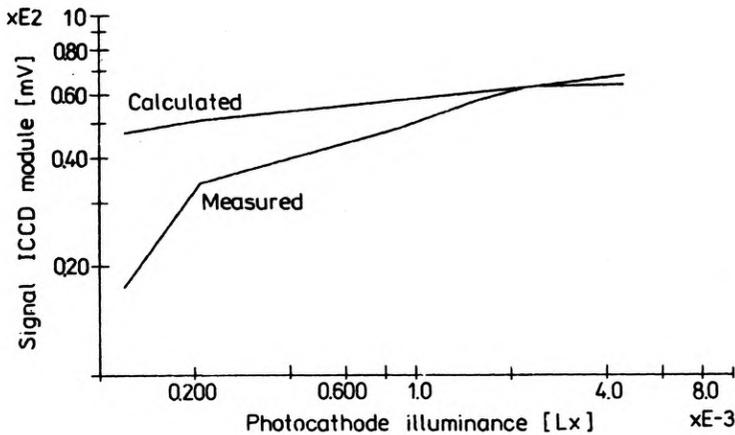
Fig. 5. Experimental measurement and theoretical prediction of ICCD modul signal against photocathode illuminance
