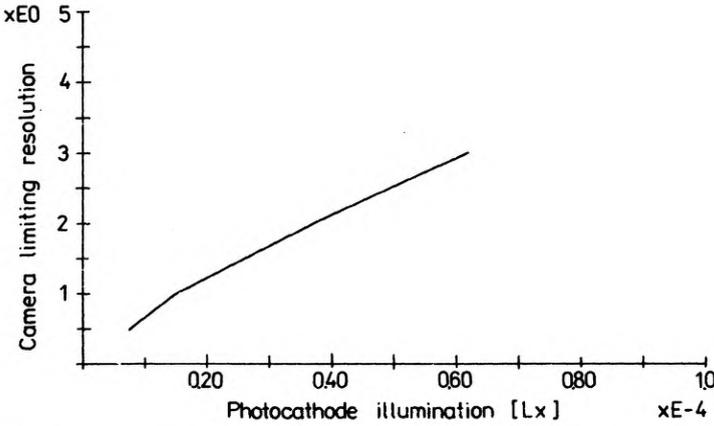
Fig. 10. Limiting resolution of ICCD camera against photocathode illumination
