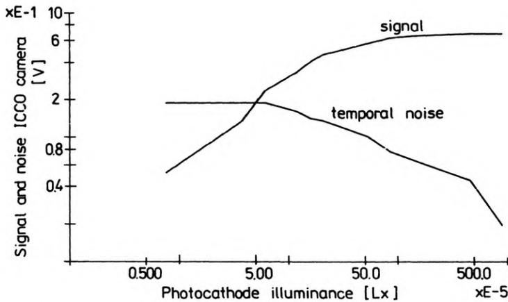
Fig. 7. Signal and noise of ICCD camera against photocathode illuminance
