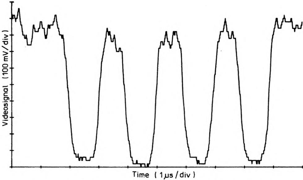
Fig. 4. Elimination of photon noise from videosignal with AVERAGING mode using TEKTRONIX 2430A digital oscilloscope
