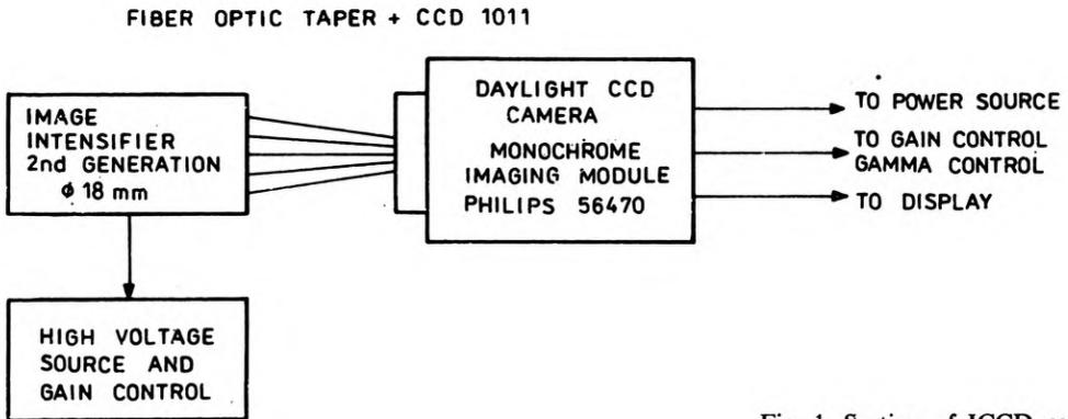
Fig. 1. Section of ICCD camera
