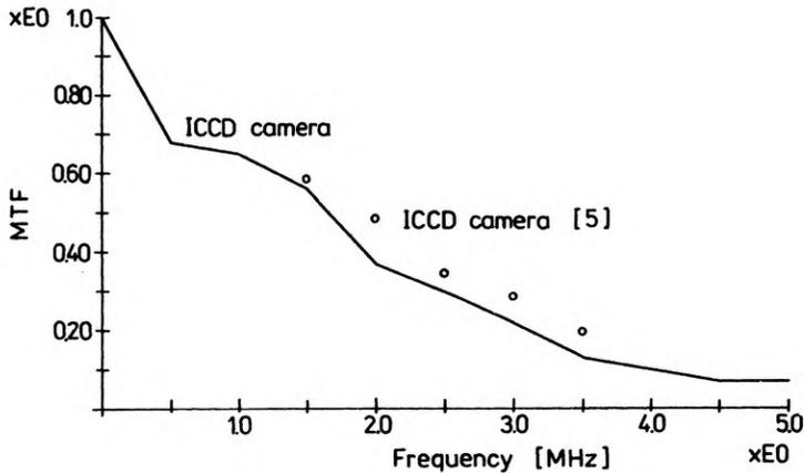
Fig. 9. MTF of ICCD camera calculated from edge response.
