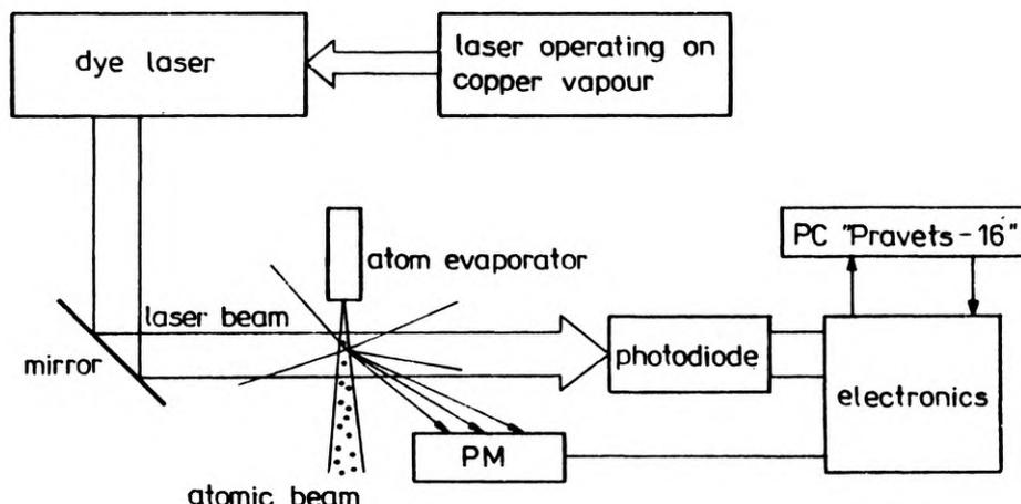
Fig. 1. Functional diagram of the laser spectroscopy
