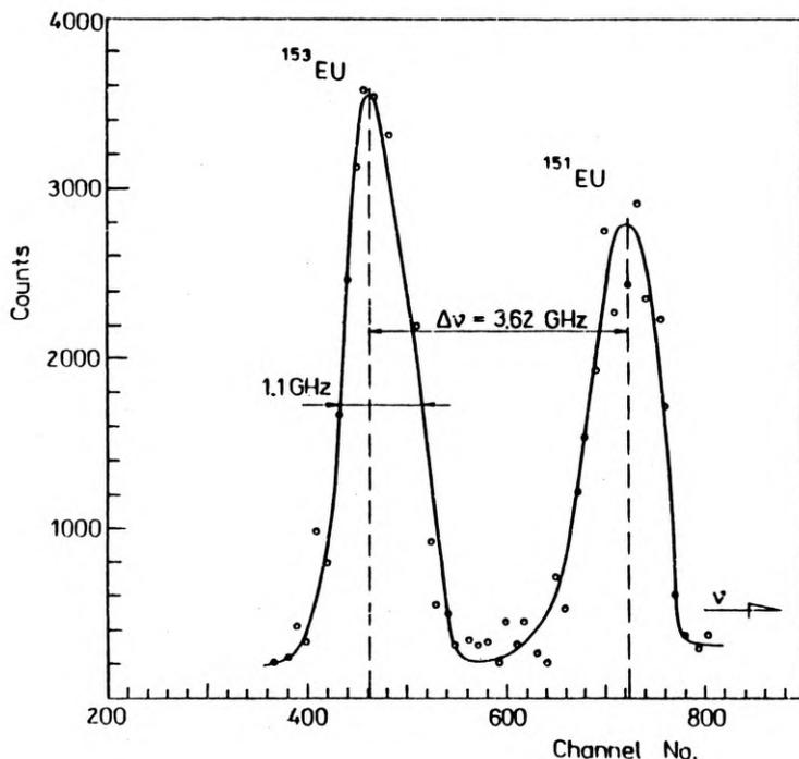
Fig. 2. Optical spectrum of natural Eu mixture, at a laser wavelength  $\lambda = 576.5 \text{ nm}$
