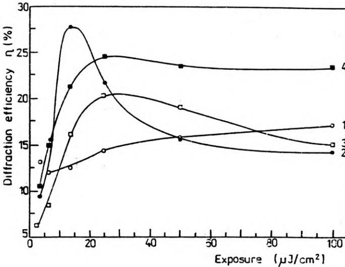
Fig. 2. Variations of the diffraction efficiency with exposure for photographic phase gratings produced with ICP 163 developer and the bleaches 1, 2, 3 and 4
