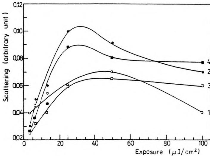
Fig. 4. Variations of scattering with exposure for photographic phase gratings produced with ICP 163 developer and the bleaches 1, 2, 3 and 4
