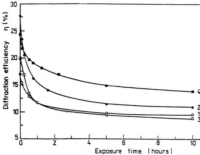
Fig. 8. Variation of the maximum diffraction efficiency as a function of exposure time (in hours) in white light of the holograms produced with ICP 163 developer and the bleaches 1, 2, 3 and 4
