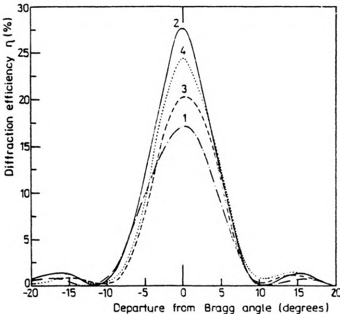
Fig. 6. Variation of the maximum diffraction efficiency as a function of departure from the Bragg angle of the holograms produced with ICP 163 developer and the bleaches 1, 2, 3 and 4
