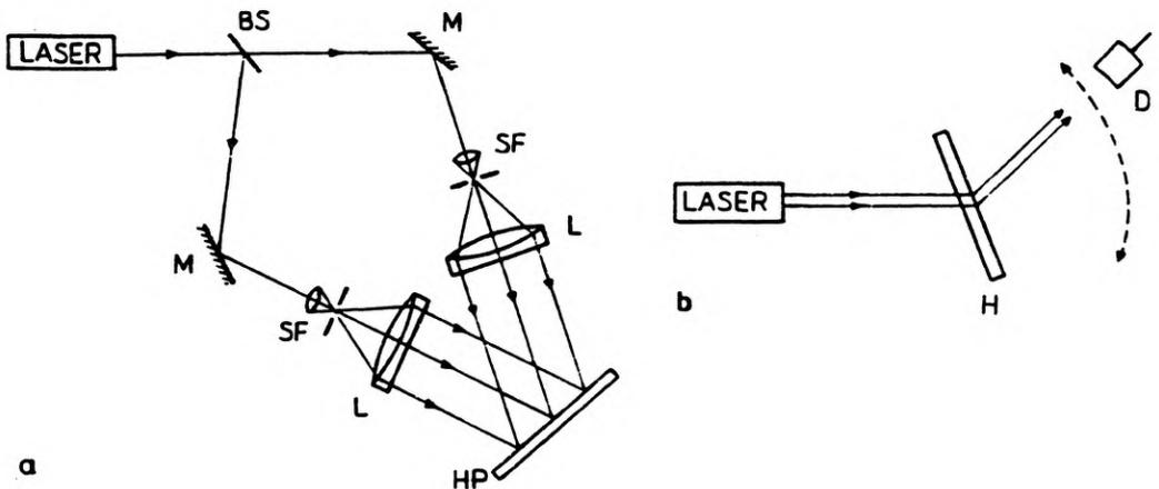
Fig. 1. Setup for recording the interference gratings (a), and setup for reconstructing the holograms and to measure the diffracted and scattered intensities (b). BS – beam splitter, M – mirror, SF – spatial filter, L – lens, HP – holographic plates, H – holograms, D – detector
