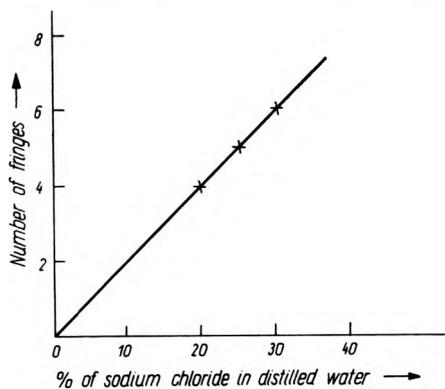
Fig. 2. Variation in number of fringes, with different concentrations of sodium chloride in distilled water
