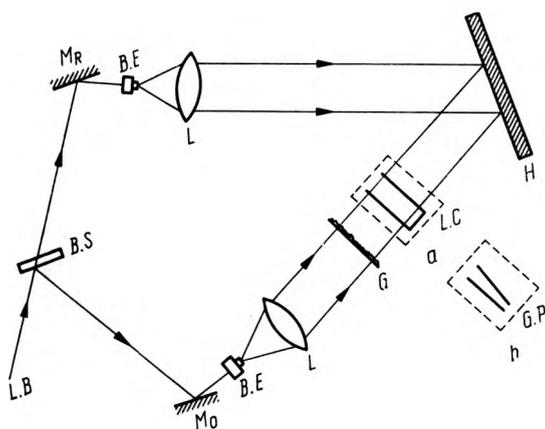
Fig. 1. Schematic diagram of the experimental set-up for making a) equal inclination fringes, and b) equal thickness fringes
