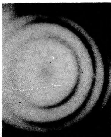
Fig. 3. Equal inclination fringes for 30% content of sodium chloride in distilled water
