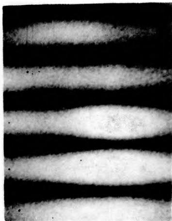
Fig. 6. Equal thickness fringes for  $0.5^\circ$  tilt between the glass plates
