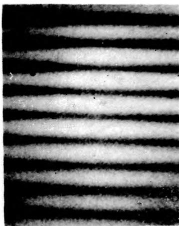
Fig. 7. Equal thickness fringes for  $1.0^\circ$  tilt between the glass plates
