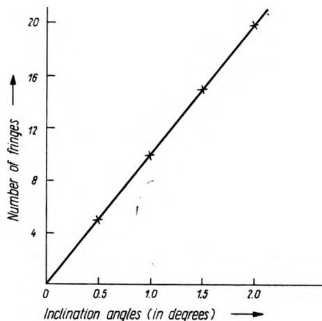
Fig. 5. Variation in number of fringes, with different angles between the glass plates
