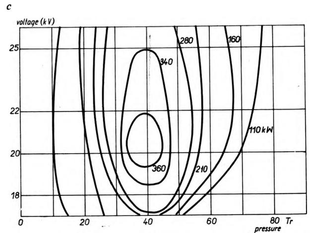
Fig. 3. Laser peak power vs. the power supply tension nitrogen pressure:
