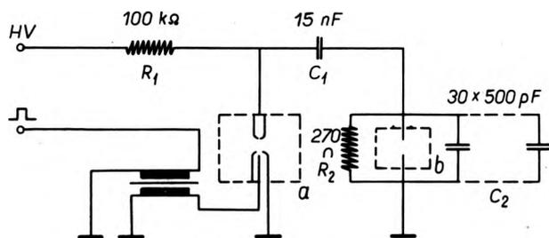
Fig. 1. Electrical circuit of the nitrogen laser
