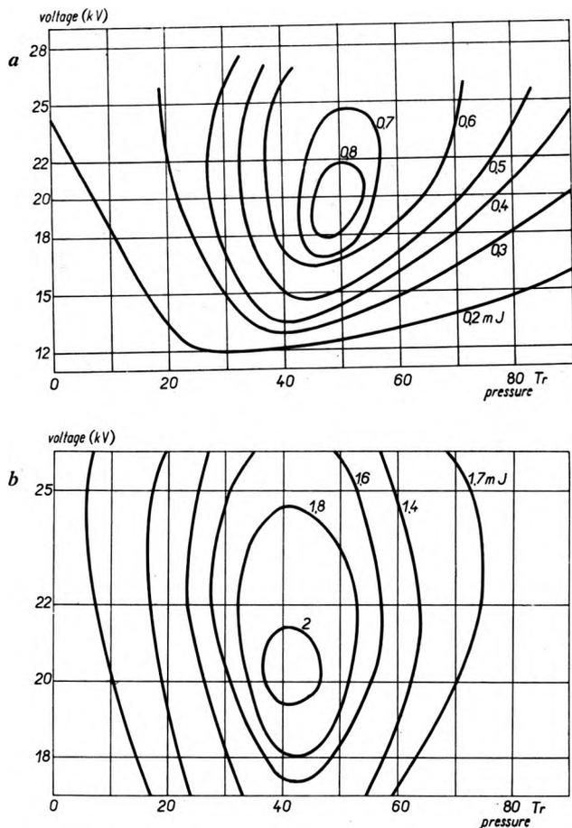
Fig. 4. Laser pulse energy vs. the power supply tension and nitrogen pressure:
