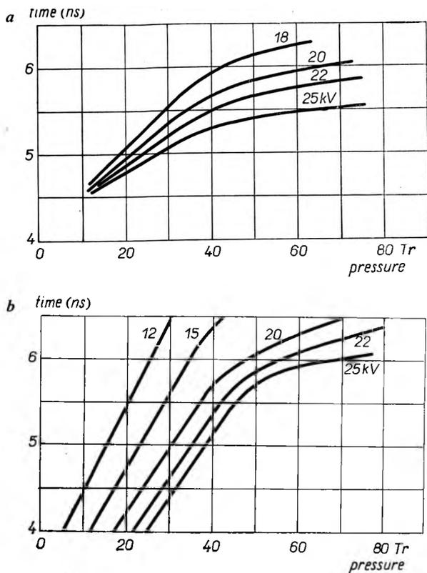
Fig. 6. Laser pulse duration (FWHM) vs. the nitrogen pressure at various power supply tensions: a - laser with one mirror, b - laser with resonator
