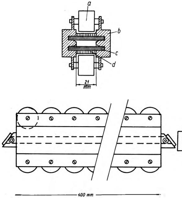
Fig. 2. Cross-section of the laser discharge channel:
