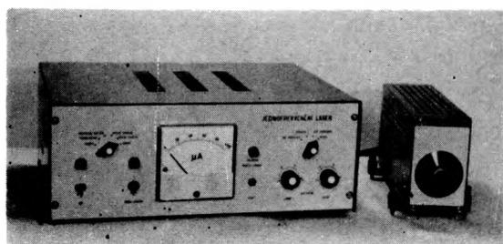
Fig. 1. Single-frequency He-Ne laser
