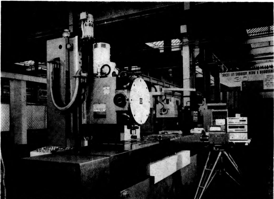
Fig. 6. Testing of an NC machine with the remote interferometer
