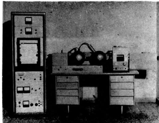
Fig. 8. Reflectometer for measuring the reflectivity and losses of laser mirrors
