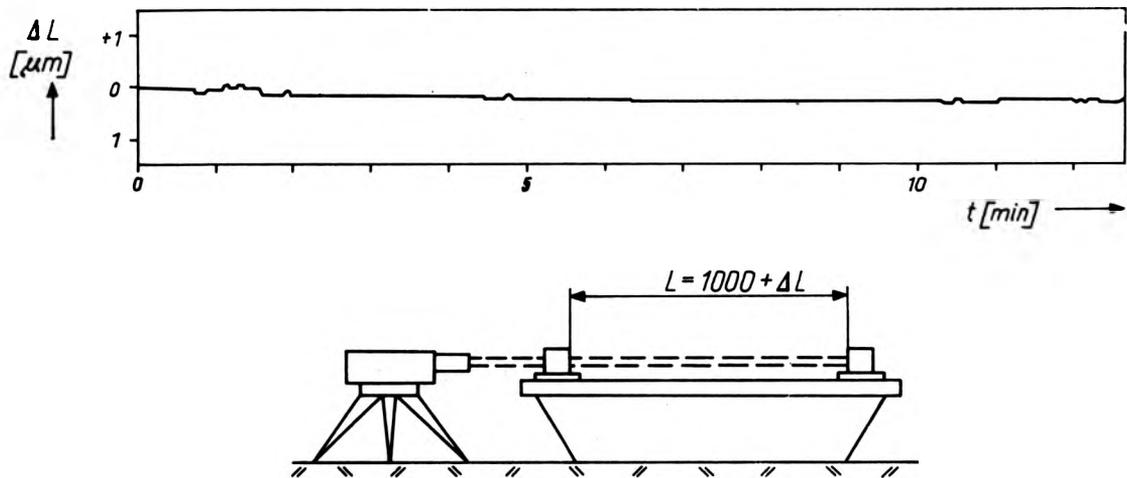
Fig. 5. Stability of the remote interferometer for working length 1 m
