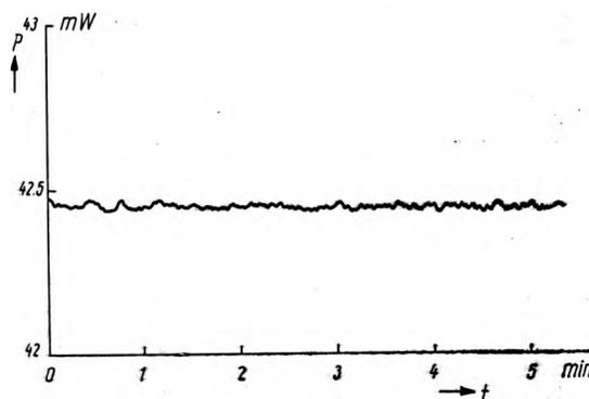
Fig. 3. Stability of the output power: laser 42.5 mW
