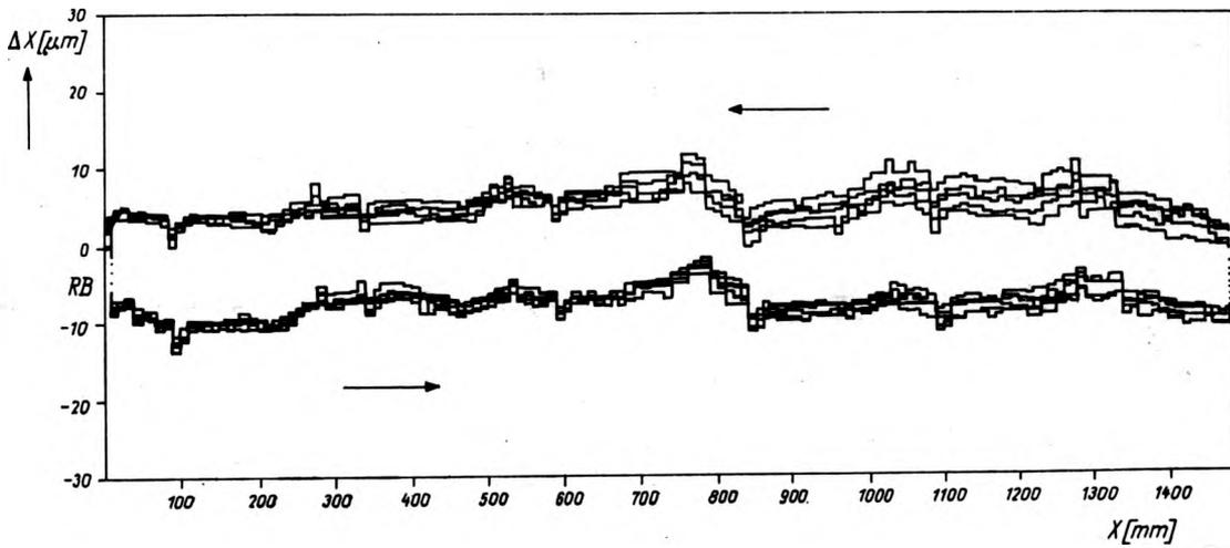
Fig. 7. Deviation record in the x-axis direction of an NC machine
