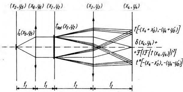
Fig. 2. Reconstruction of Fourier-type hologram
