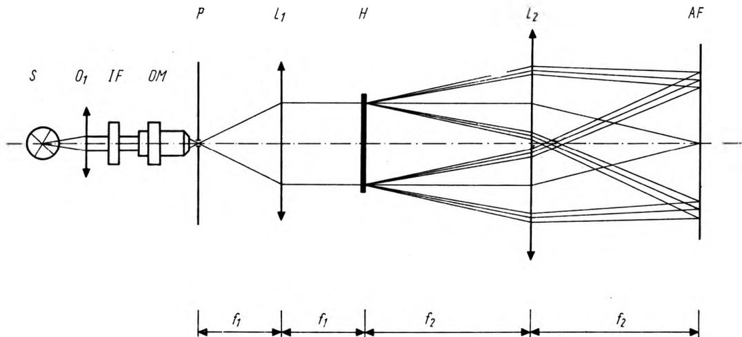
Fig. 3. Diagram of an experimental setup for partially coherent reconstruction of Fourier holograms
