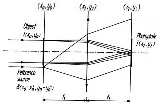
Fig. 1. Recording of Fourier-type hologram
