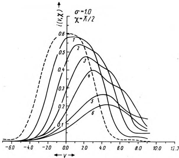
Fig. 6. Diffraction images of an incoherent annulus for different amount of aberration (dotted curve shows the aberration free case for  $\sigma = 1.0$  and  $\chi = \pi/2$
