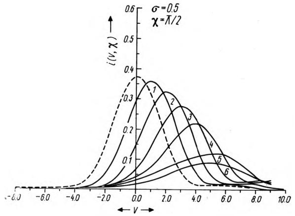
Fig. 3. Diffraction images of an incoherent annulus for different amount of aberration (dotted curve shows the aberration free case) for  $\sigma = 0.5$  and  $\chi = \pi/2$
