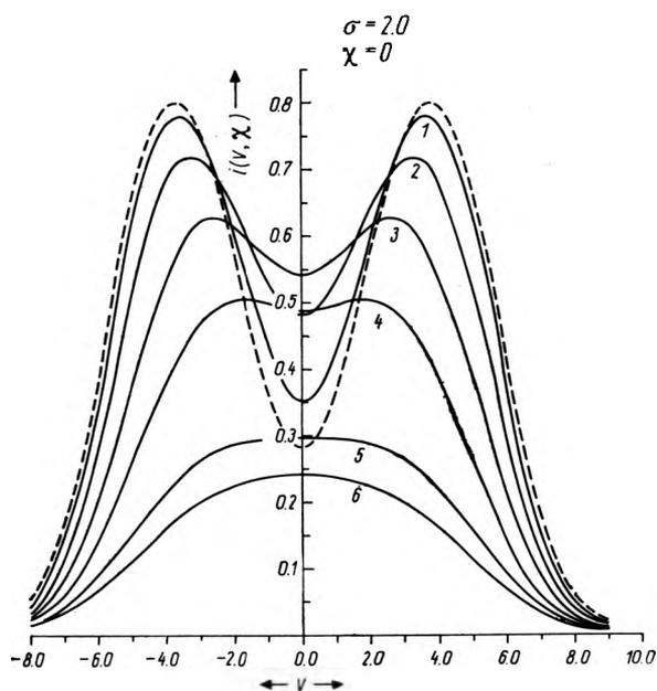
Fig. 10. Diffraction images of an incoherent annulus for different amount of aberration (dotted curve shows the aberration free case) for  $\sigma = 2.0$  and  $\chi = 0$
