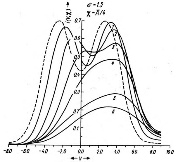
Fig. 8. Diffraction images of an incoherent annulus for different amount of aberration (dotted curve shows the aberration free case for  $\sigma = 1.5$  and  $\chi = \pi/4$
