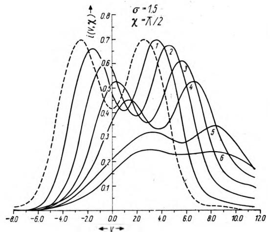
Fig. 9. Diffraction images of an incoherent annulus for different amount of aberration (dotted curve shows the aberration free case for  $\sigma = 1.5$  and  $\chi = \pi/2$
