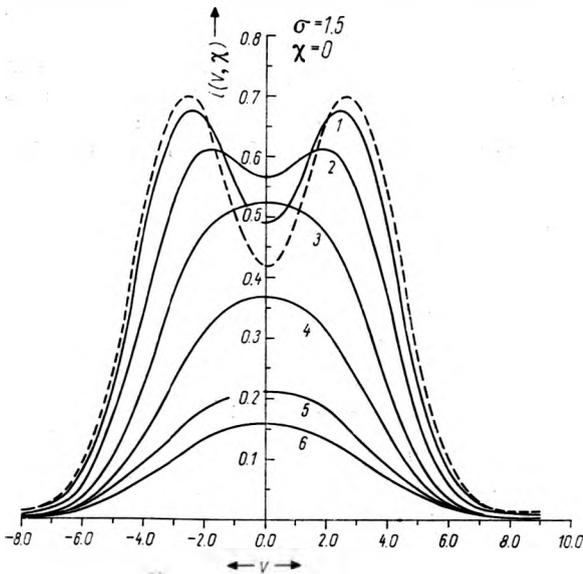
Fig. 7. Diffraction images of an incoherent annulus for different amount of aberration (dotted curve shows the aberration free case for  $\sigma = 1.5$  and  $\chi = 0$
