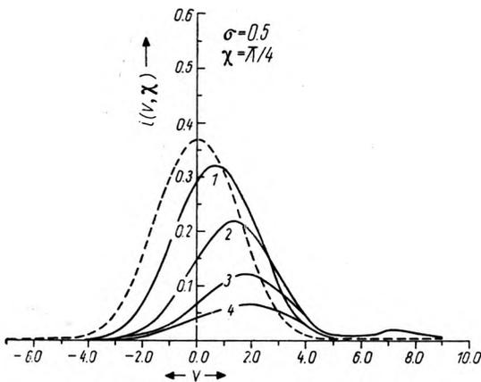
Fig. 2. Diffraction images of an incoherent annulus for different amount of aberration (dotted curve shows the aberration free case) for  $\sigma = 0.5$  and  $\chi = \pi/4$
