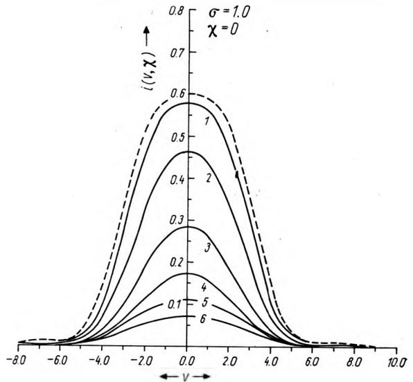
Fig. 4. Diffraction images of an incoherent annulus for different amount of aberration (dotted curve shows the aberration free case) for  $\sigma = 1.0$  and  $\chi = 0$
