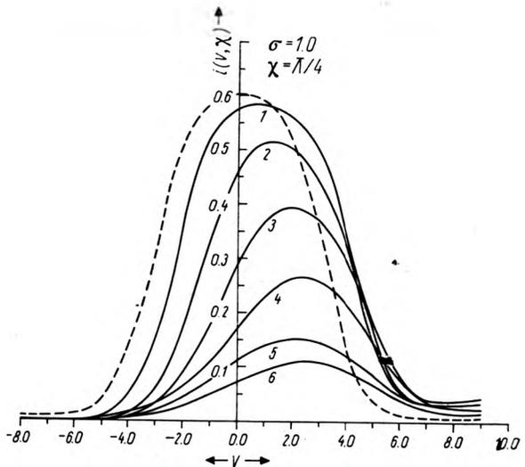
Fig. 5. Diffraction images of an incoherent annulus for different amount of aberration (dotted curve shows the aberration free case) for  $\sigma = 1.0$  and  $\chi = \pi/4$
