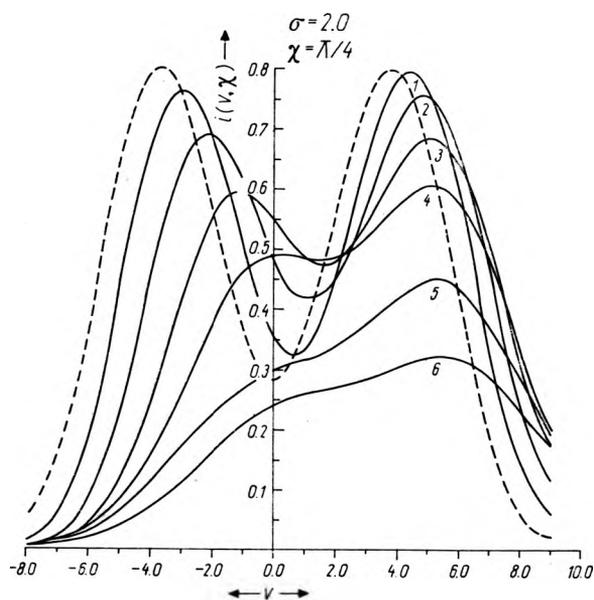
Fig. 11. Diffraction images of an incoherent annulus for different amount of aberration (dotted curve shows the aberration free case) for  $\sigma = 2.0$  and  $\chi = \pi/4$
