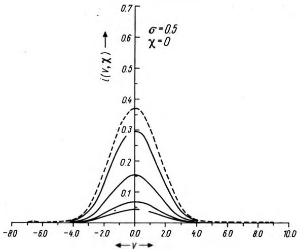
Fig. 1. Diffraction images of an incoherent annulus for different amount of aberration (dotted curve shows the aberration free case) for  $\sigma = 0.5$  and  $\chi = 0$
