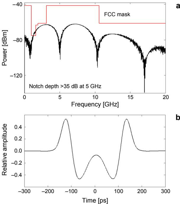
Fig. 3. The generated UWB signals with a spectral notch-band at 5GHz. Signal power spectrum (a), and UWB signal waveform (b).
