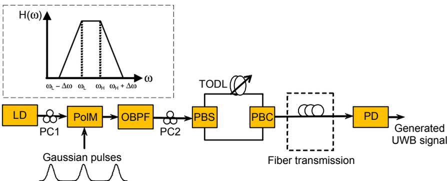
Fig. 1. Schematic diagram of the proposed UWB signal generation system. LD – laser diode, PoIM – polarization modulator, OBPF – optical bandpass filter, PBS – polarization beam splitter, PBC – polarization beam combiner, PC – polarization controller, TODL – tunable optical delay line, PD – photodetector; insert – ideal response of an OBPF.
