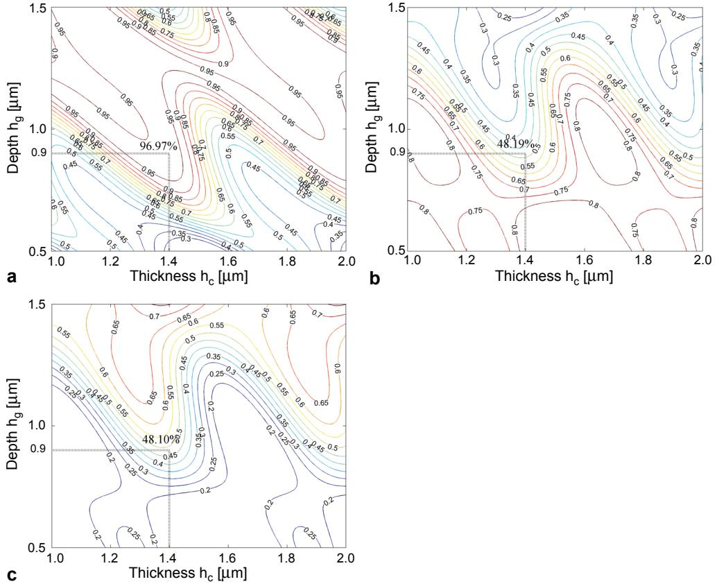
Fig. 2. Reflection efficiency versus grating depth and thickness of the connecting layer with the duty cycle of 0.5 and period of 1181 nm for the wavelength of 1550 nm: TE polarization diffracted into the  $-1^{\text{st}}$  order (**a**), TM polarization diffracted into the 0th order (**b**), and TM polarization diffracted into the  $-1^{\text{st}}$  order (**c**).
