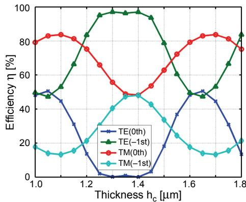
Fig. 3. Reflection efficiency versus thickness of the connecting layer with the duty cycle of 0.5, period of 1181 nm and depth of 0.90 μm for the wavelength of 1550 nm under the Littrow mounting.
