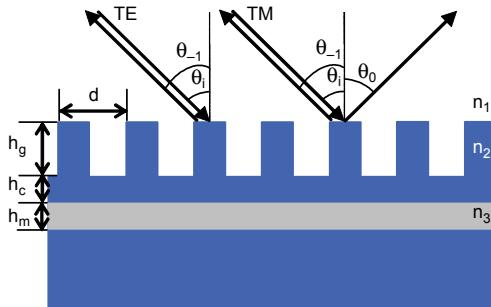
Fig. 1. Schematic of a reflective dual-function grating by a metal-mirror-based grating (refractive indices  $n_1$  – air,  $n_2$  – fused silica,  $n_3$  – Ag;  $d$  – period;  $h_g$  – grating depth,  $h_c$  and  $h_m$  – thickness of the connecting layer and metal slab, respectively;  $\theta_i$  – incident angle,  $\theta_{-1}$  and  $\theta_0$  – diffraction angles of the  $-1$ st and  $0$ th orders, respectively).
