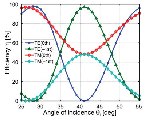
Fig. 5. Reflection efficiency versus angle of incidence for the wavelength of 1550 nm with the optimized grating profile parameters.
