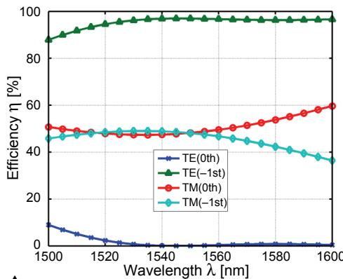
Fig. 4. Reflection efficiency versus incident wavelength under the Littrow mounting with the optimized grating parameters.
