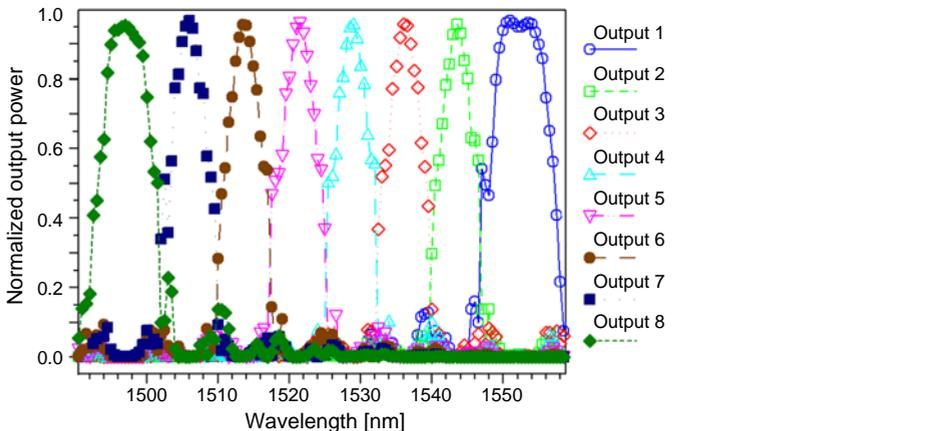
Fig. 6. Output spectral transmission of the proposed structure in first state.
