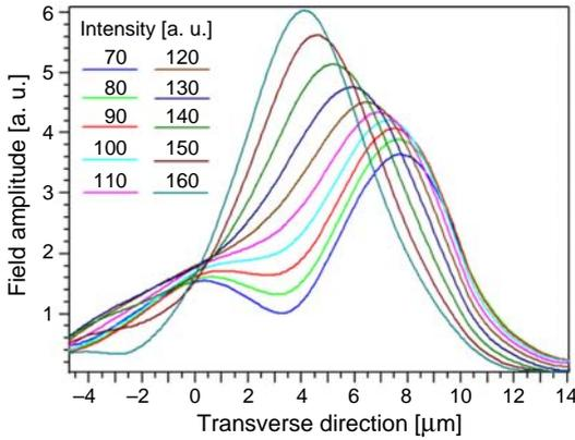
Fig. 3. Effect of changing intensity on field profile distribution in length  $L_x$ .
