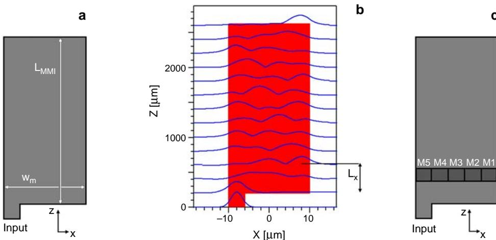
Fig. 1. Basic structure of multimode interference devices (a). Beam propagation simulation of the structure in linear state (input intensity is low) (b). Structure with five power monitors for the simulation of the specified region (c).
