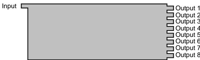
Fig. 4. The proposed structure for 1×8 multimode interference switch.
