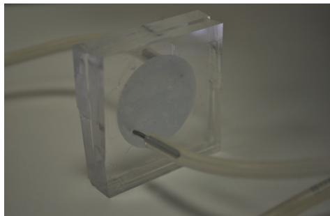
Fig. 6. PDMS pre-concentrator with polycarbonate filtration membrane and microfluidic connectors.
