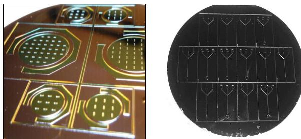
Fig. 4. Masters of a pre-concentrator and microfluidic chip, with negative patterns of microchannels made in UV-curable epoxy resin SU-8.
