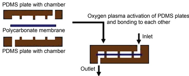
Fig. 7. Method of fixing of polycarbonate membrane inside the pre-concentrator.
