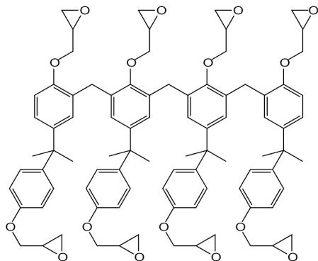
Fig. 3. Structural formula of the SU-8 resin.
