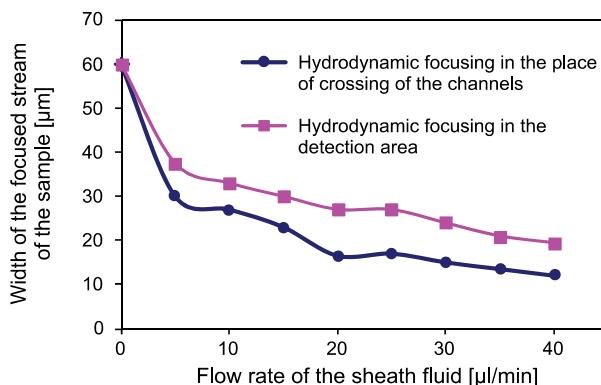
Fig. 10. Relationship between flow rate of sheath fluid and width of the central fluid stream after hydrodynamic focusing; flow rate of the central fluid – 10  $\mu\text{l}/\text{min}$ .
