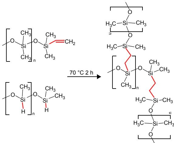
Fig. 5. Crosslinking reaction between PDMS monomer and curing agent.
