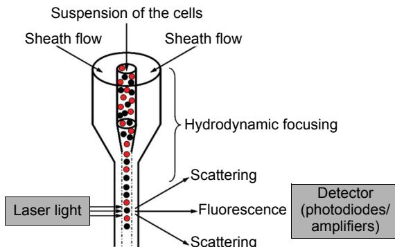
Fig. 1. The principle of operation of flow cytometry.
