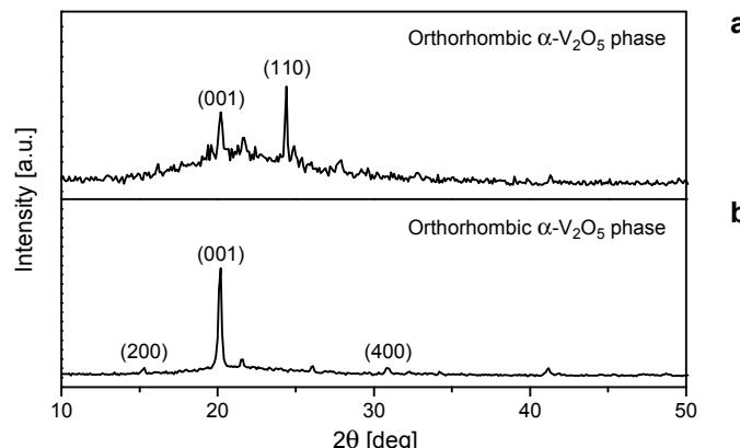
Fig. 1. XRD patterns of annealed (400 °C) vanadium oxides deposited at:  $3 \times 10^{-4}$  Torr (a) and  $7 \times 10^{-4}$  Torr (b) of oxygen partial pressure.
