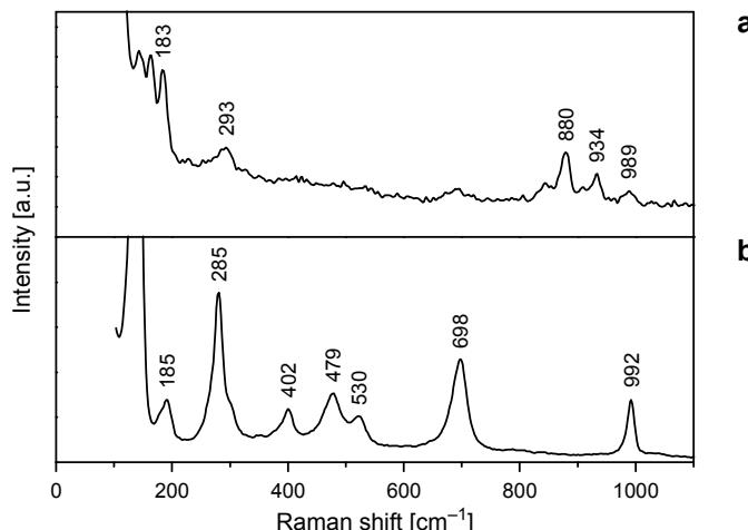
Fig. 2. Raman spectra of annealed ( $400^\circ\text{C}$ ) vanadium oxide thin films prepared with different partial pressure of  $O_2$ :  $3 \times 10^{-4}$  Torr (a), and  $7 \times 10^{-4}$  Torr (b). Used laser excitation was 476.5 nm.
