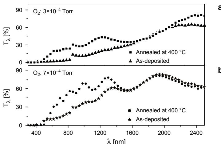
Fig. 3. Optical transmission spectra of as-deposited and annealed (400 °C) vanadium oxide thin films prepared in different partial pressure of O<sub>2</sub>: 3×10<sup>-4</sup> Torr (a), and 7×10<sup>-4</sup> Torr (b).
