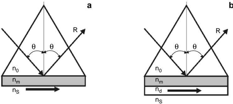
Fig. 1. The prismatic structures of the plasmon polariton (a) and waveguide (b) resonances, where  $n_0$  – refractive index of prism,  $n_m$  – refractive index of metallic film,  $n_s$  – refractive index of surrounding media,  $n_d$  – refractive index of dielectric film,  $R$  – reflectivity.
