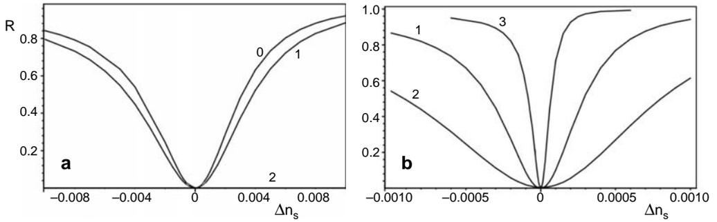
Fig. 5. Dependence of reflectivity on refractive index of the liquid: TM polarization (a), TE polarization (b).
