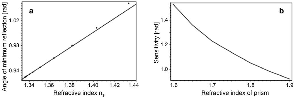
Fig. 4. Dependence of the minimum reflectivity on the analyzed liquid refractive index (a) and dependence of the sensitivity  $S_m$  on the prism refractive index  $n_0$  (b).
