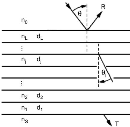
Fig. 2. Composition of multilayer structure.
