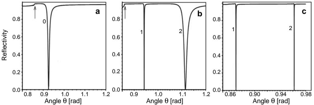
Fig. 3. Reflectivity vs. laser beam angle of incidence at the metal film: TM polarization, dielectric thickness equals zero (a), TM polarization, dielectric thickness is  $0.8 \mu\text{m}$  (b), TE polarization, dielectric thickness is  $0.8 \mu\text{m}$  (c).
