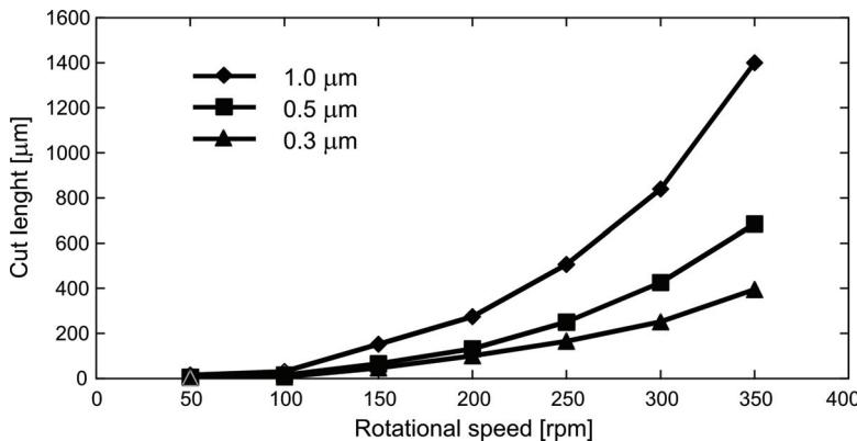
Fig. 1. Graph of cut off length *vs.* rotational speed using sandpaper of size 1.0  $\mu\text{m}$ , 0.5  $\mu\text{m}$  and 0.3  $\mu\text{m}$ . The equation of the curve  $y = 0.0041x^2 - 0.3352x$ .
