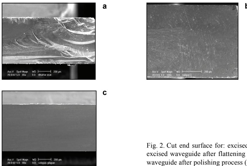
Fig. 2. Cut end surface for: excised waveguide (a), excised waveguide after flattening (b), and excised waveguide after polishing process (c).
