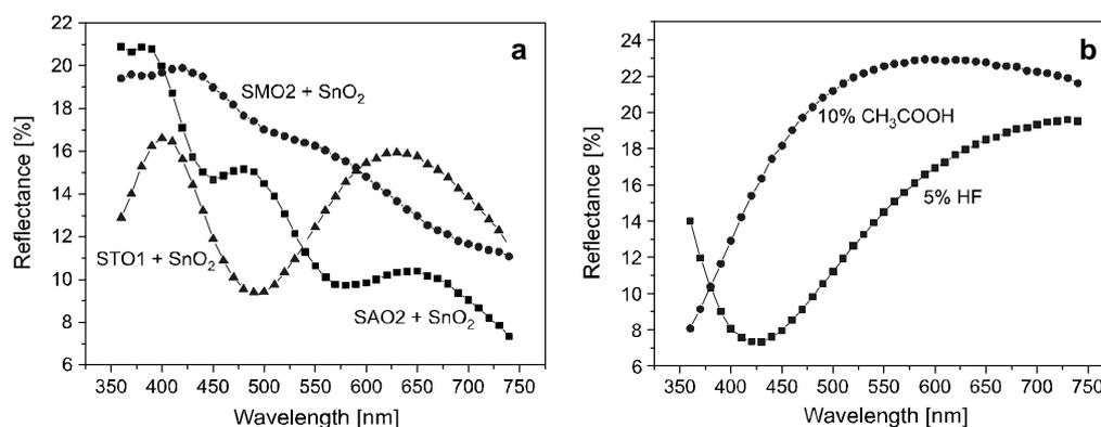
Fig. 3. Reflectance as a function of wavelength: **a** – SnO<sub>2</sub> thin film on glasses with different sodium diffusion barrier coatings, **b** – SnO<sub>2</sub> thin film on glasses treated in fluoric and acetic acid.
