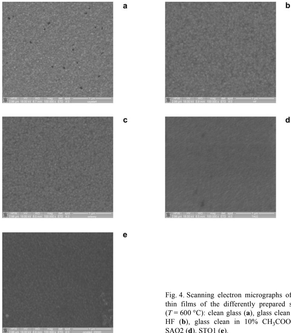
Fig. 4. Scanning electron micrographs of  $\text{SnO}_2$  thin films of the differently prepared surface ( $T = 600^\circ\text{C}$ ): clean glass (a), glass clean in 5% HF (b), glass clean in 10%  $\text{CH}_3\text{COOH}$  (c),  $\text{SAO}_2$  (d),  $\text{STO1}$  (e).
