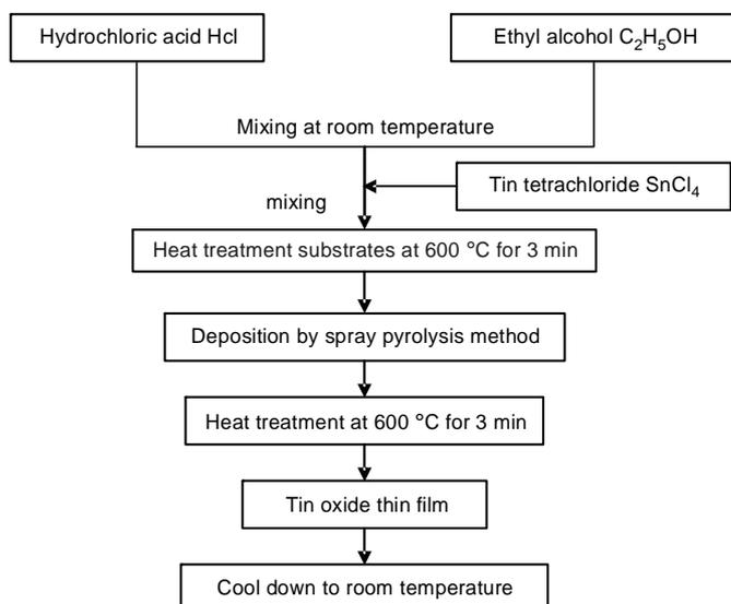
Fig. 1. Preparation procedure of a thin film by the spray pyrolysis process.
