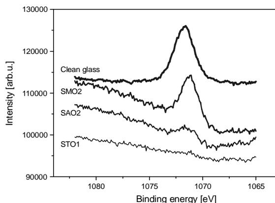
Fig. 2. XPS spectra – Na 1s region. Comparison of Na 1s peak for clean glass and SnO<sub>2</sub> coated samples.
