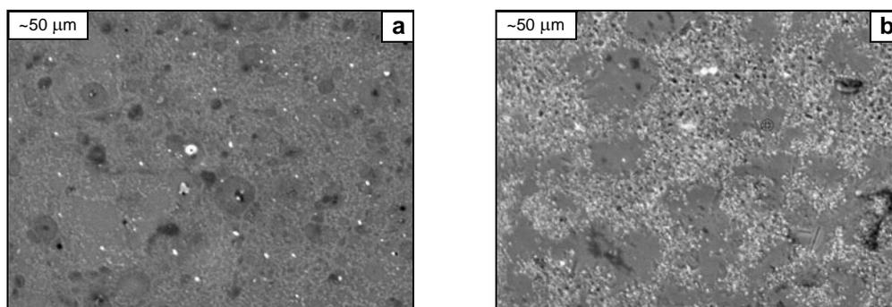
Fig. 5. Microstructure of G78 sample; **a** – after firing, **b** – after corrosion in 1% citric acid.
