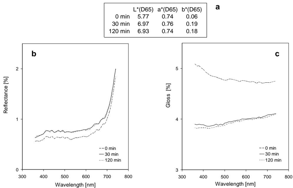
Fig. 2. Spectral characteristic of G205 coating coloured by pigment after corrosion in 1% sulfur acid; **a** – colour parameters, **b** – reflectance, **c** – gloss.
