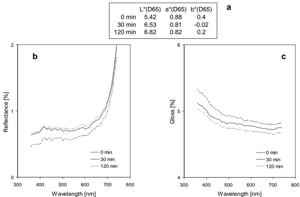
Fig. 4. Spectral characteristic of G205 coating coloured by pigment after corrosion in 0.5% NaOH; **a** – colour parameters, **b** – reflectance, **c** – gloss.
