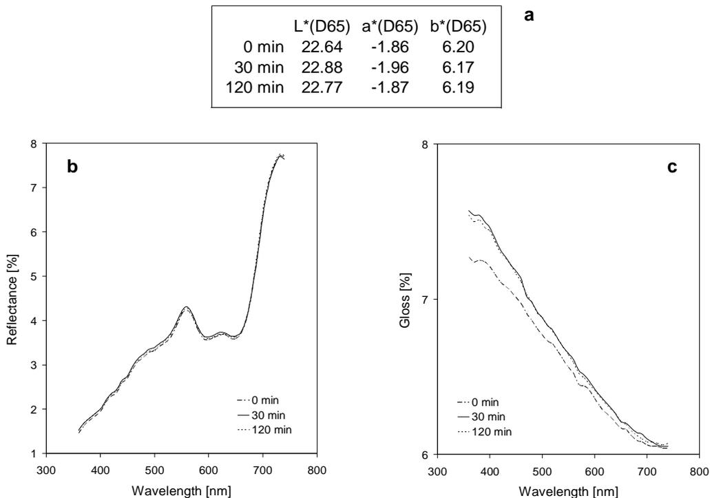
Fig. 1. Spectral characteristic of G102 coating (ion pigmented) after corrosion in 1% sulfur acid; **a** – colour parameters, **b** – reflectance, **c** – gloss.
