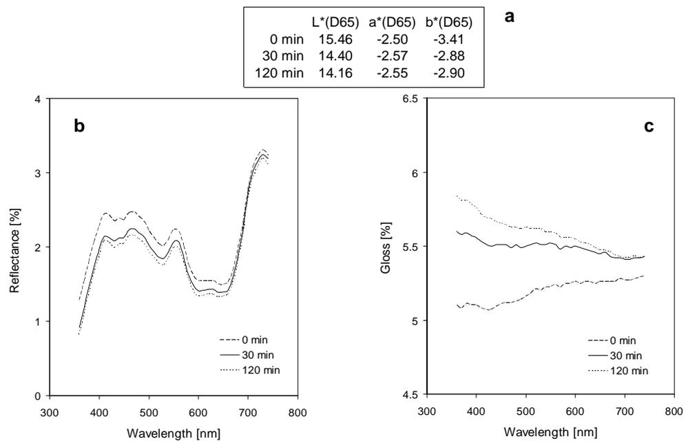
Fig. 3. Spectral characteristic of G107 coating (ion pigmented) after corrosion in 1% NaOH; **a** – colour parameters, **b** – reflectance, **c** – gloss.
