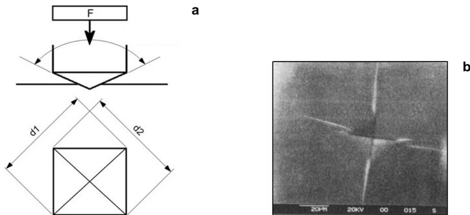
Fig. 2. Schematic presentation of the Vickers indentation (a) and the cracks appearing around (b).
