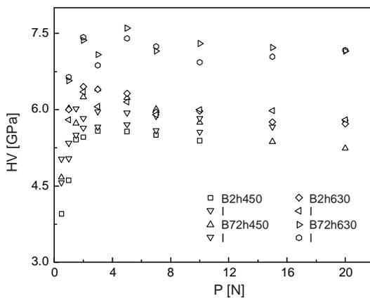
Fig. 4. Load dependence of microhardness of samples exchanged for two and 72 h at 723 K and 903 K as well as for those hydrogenated afterwards.
