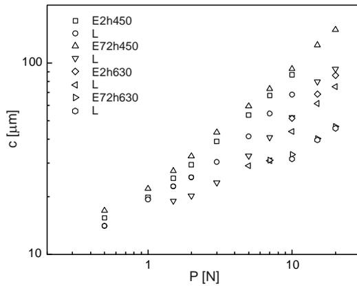
Fig. 3. Load dependence of the length of cracks (in a double logarithmic presentation) formed around the Vickers indentation mark in specimens exchanged with copper at high and low temperature for two and 72 h and for the afterwards hydrogenated samples.
