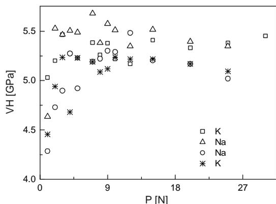
Fig. 5. Load dependence of microhardness of some SLS glasses containing different amounts of sodium and potassium oxide.
