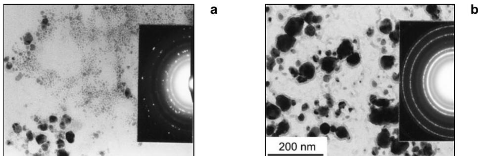
Fig. 1. TEM micrographs of SLS glass specimens exchanged at 723 K (a) and 903 K (b).
