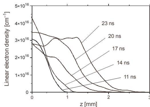
Fig. 7. Diagrams of the linear electron density of the axial plasma stream at different instants of its propagation.
