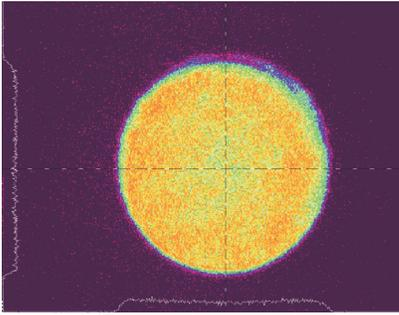
Fig. 2. Typical intensity distribution in the laser beam cross-section.
