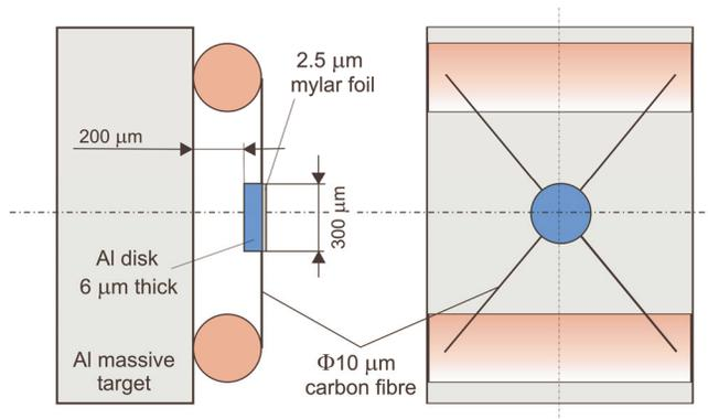
Fig. 3. Construction of the double target.
