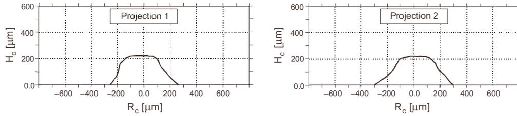
Fig. 4. Shapes and dimensions of the crater (in two mutually perpendicular projections) produced by the flyer disk, where:  $R_c$  and  $H_c$  are the radius and the depth of the crater, respectively.
