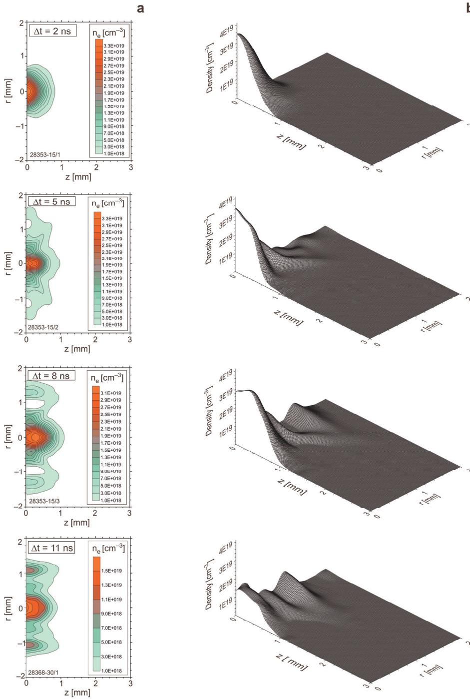
Fig. 5. A sequence of electron isodensitygrams (a) and electron density distributions (b) corresponds to the appearance and decay of ablative plasma.
