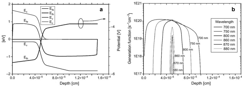
Fig. 5. Band-gap diagram (a) and generation function (b) of wavelength sensitive photodetector with graded emitter.
