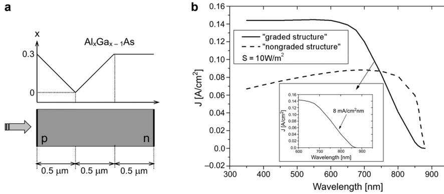
Fig. 2. Scheme of the wavelength sensitive photodetector (a), spectral sensitivity of structure with graded and non-graded emitter (b).
