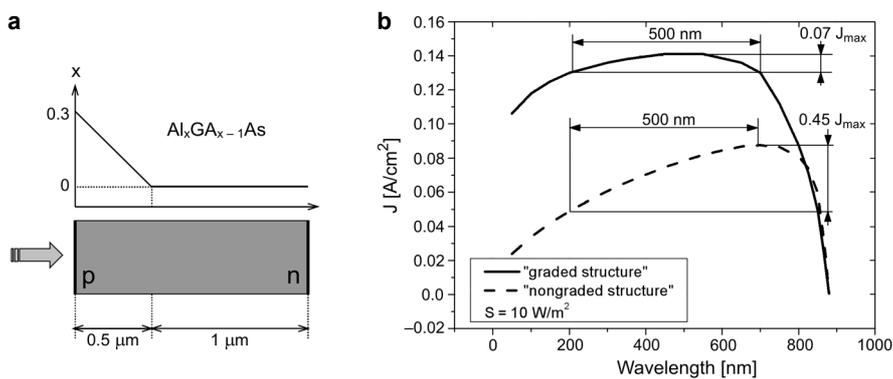
Fig. 1. Scheme of the active area of *p*-*n* photodetector with graded emitter (a) and comparison of spectral sensitivity of detectors with graded and non-graded emitter (b).
