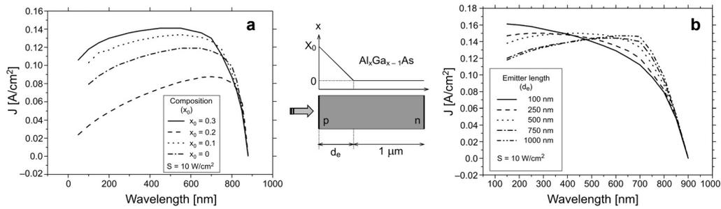
Fig. 3. The dependence of spectral characteristics of  $p-n$  photodetector with graded emitter vs. emitter: composition (a) and length (b).
