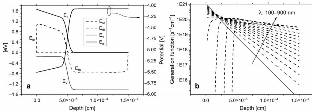
Fig. 4. Band-gap diagram (a) and generation function (b) of *p-n* photodetector with graded emitter.
