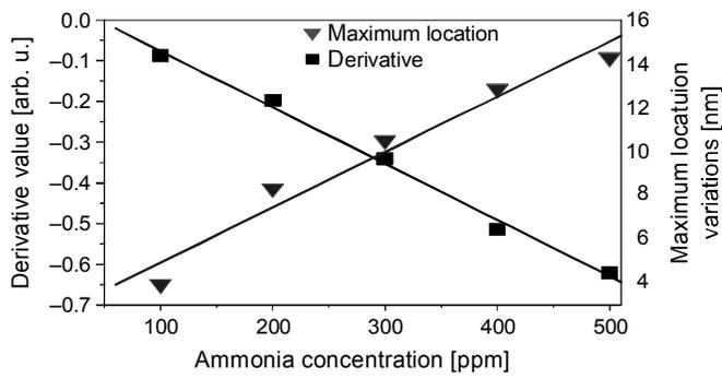
Fig. 8. Linear dependence of maximum location changes and its derivative versus ammonia concentration.
