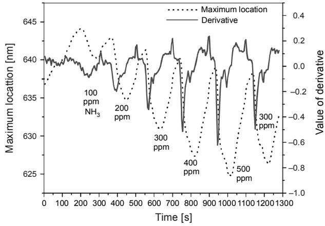
Fig. 7. Response to various  $\text{NH}_3$  concentrations at 75% humidity level.
