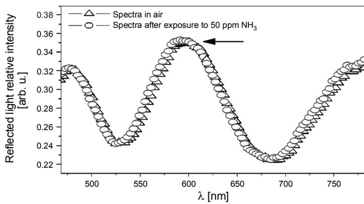
Fig. 2. The example of maximum location upon NH<sub>3</sub> exposure.
