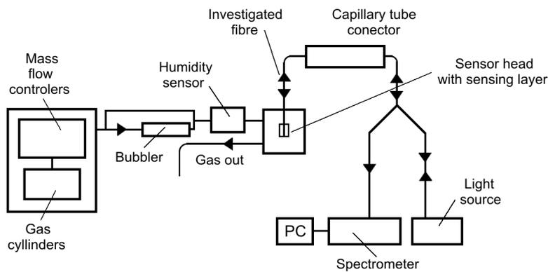
Fig. 3. The measuring setup.
