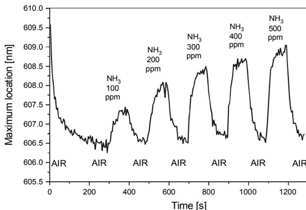
Fig. 4. Response to various NH<sub>3</sub> concentrations at low humidity level.
