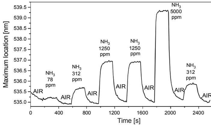
Fig. 5. Response to various  $\text{NH}_3$  concentrations at low humidity level.
