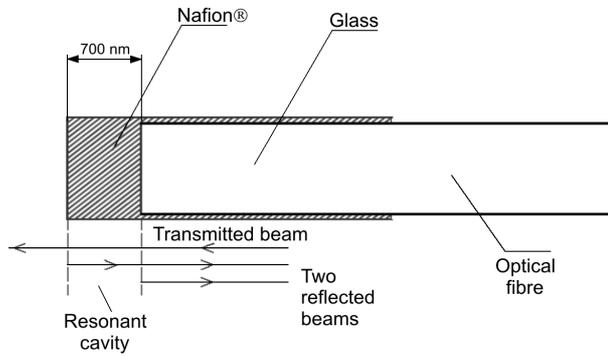
Fig. 1. The sensor head.
