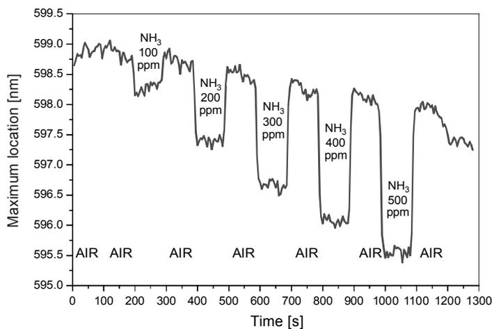
Fig. 6. Response to various  $\text{NH}_3$  concentrations at 35% humidity level.
