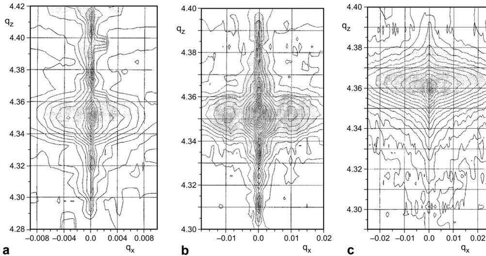
Fig. 4. Reciprocal lattice maps of  $\text{In}_{0.13}\text{Ga}_{0.87}\text{As}$  layers: 30 nm (a), 58 nm (b), and 80 nm (c).
