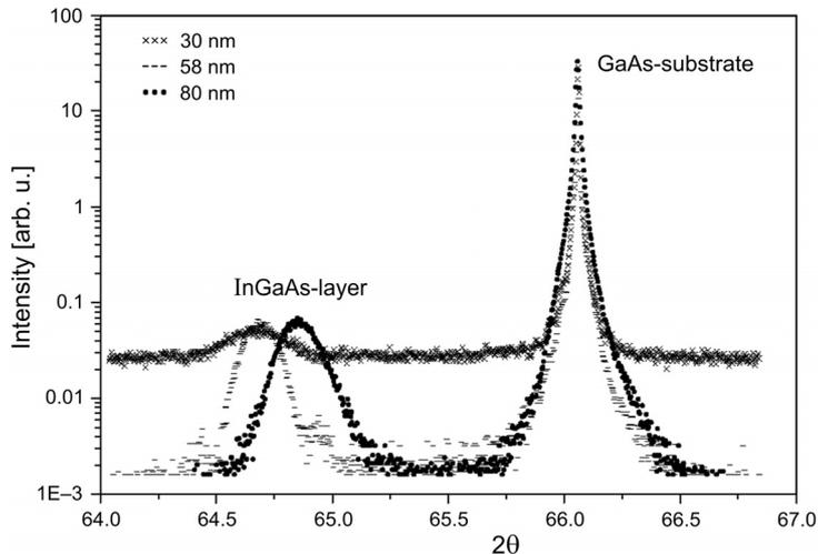
Fig. 3. HR XRD (004) rocking curves for three thickness values of  $\text{In}_{0.13}\text{Ga}_{0.87}\text{As}$  layers: 30 nm, 58 nm, and 80 nm.
