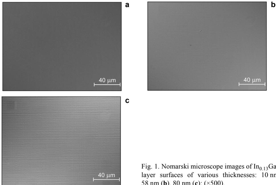
Fig. 1. Nomarski microscope images of  $\text{In}_{0.13}\text{Ga}_{0.87}\text{As}$  layer surfaces of various thicknesses: 10 nm (a), 58 nm (b), 80 nm (c); ( $\times 500$ ).
