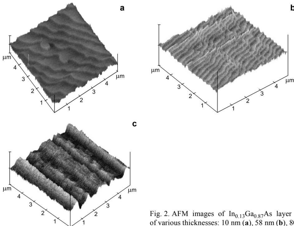
Fig. 2. AFM images of  $\text{In}_{0.13}\text{Ga}_{0.87}\text{As}$  layer surfaces of various thicknesses: 10 nm (a), 58 nm (b), 80 nm (c).
